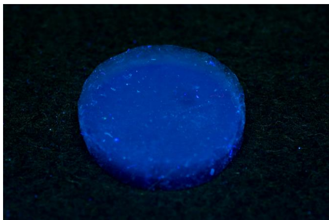
Figure S4. Photoluminescence (excited at \lambda = 254 nm) of the \gamma - \text{Al}_2\text{O}_3 monolith derived from the BNF aerogel (30 mm in diameter and 5 mm height).
