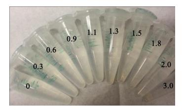
**Figure S2.** Phase behavior of PAA/PDMAEMA mixtures with equi-molar concentrations of monomers at pH 3 and room temperature. Numbers indicate the KCl concentration in moles, M.
