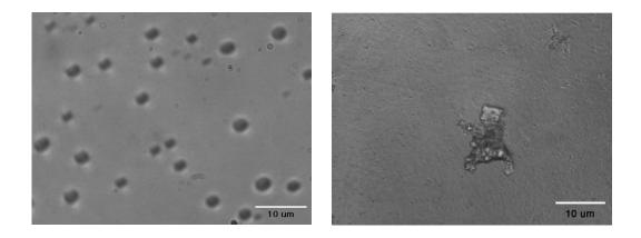
**Figure S3.** Typical optical micrographs used in distinguishing a coacervate phase from a precipitate phase for PAA/PDMAEMA at pH 7 at 900 mM KCl salt (left), and PAA/PDMAEMA at pH 5 at 300 mM KCl salt (right).
