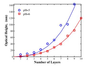
**Figure S1.** Ellipsometry measurements of film height for PAA/PDMAEMA LbL layers at room temperature in the absence of salt.
