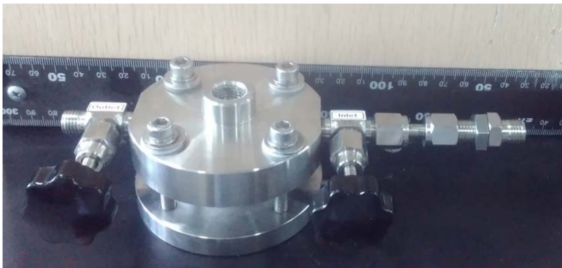
Figure S5. The gas-tight zinc-air battery for the measurement of the electrolyte decomposition. The gas evolution is measured by gas chromatography (GC7980) with thermal conductivity detection (TCD).
