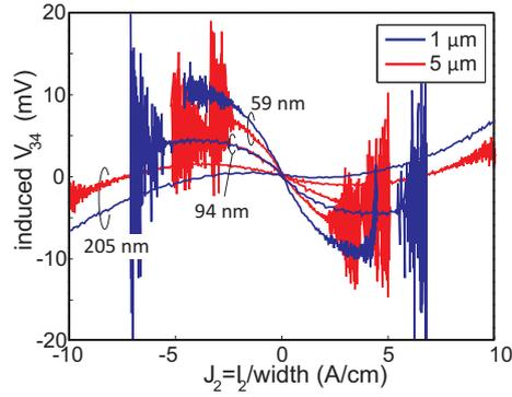
FIG. 2. Induced voltage  $V_{34}$  versus current density  $J_2$  for  $1 \mu\text{m}$  (blue) and  $5 \mu\text{m}$ -long (red) crosses on InAlN/GaN heterostructure at 4 K.
