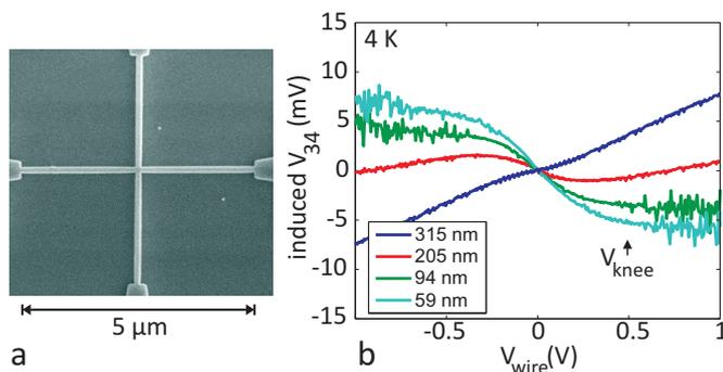
FIG. 1. Induced voltage  $V_{34}$  versus applied voltage  $V_{\text{wire}}$  for 5  $\mu\text{m}$ -long crosses on InAlN/GaN heterostructure. (a) SEM images of 5  $\mu\text{m}$ -long nanoscale crosses. (b) Measurement at 4 K showing again a change from drift (positive slope) to ballistic transport (negative slope) as the cross width is reduced. However, a much less pronounced ballistic effect is observed for these longer crosses as well as a much larger  $V_{\text{knee}}$ , close to 500 mV.
