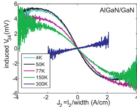
FIG. 3. Induced voltage  $V_{34}$  versus  $J_2$ , for a  $1 \mu\text{m}$ -long and  $98 \text{ nm}$ -wide cross on AlGaN/GaN heterostructures for temperatures varying from 300 K to 4 K.
