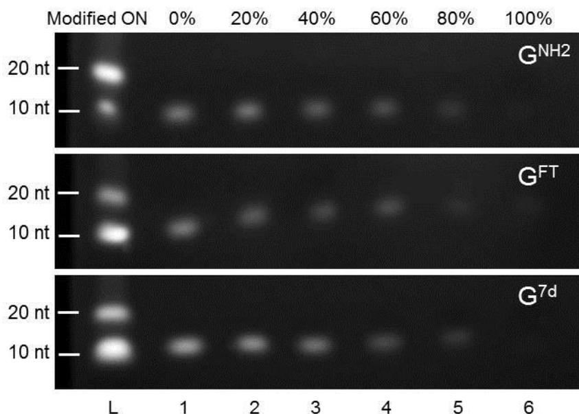
**Figure S2.** Analysis of GelRed fluorescence quenching of NEAR products on agarose gels. Each line contains the same amount of DNA, but the ratio of non-modified (containing natural  $dG$ ) and modified (containing  $dG^{NH_2}$ ,  $dG^{FT}$ , or  $dG^{7d}$ ) varies. L = DNA ladder. Lane 1: 100% natural; lane 2: 80% natural; lane 3: 60% natural; lane 4: 40% natural; lane 5: 20% natural; lane 6: 0% natural.
