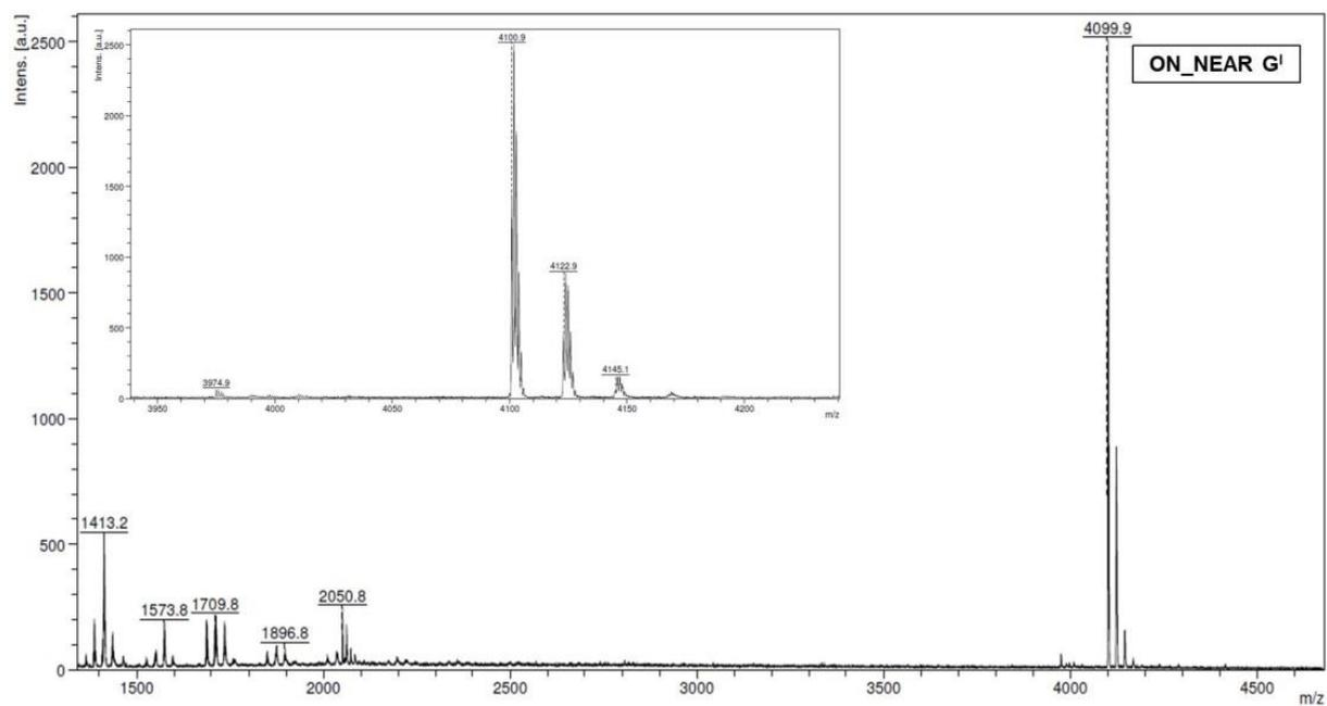
**Figure S12.** MALDI-TOF spectrum of **ON\_NEAR G<sup>I</sup>**.
