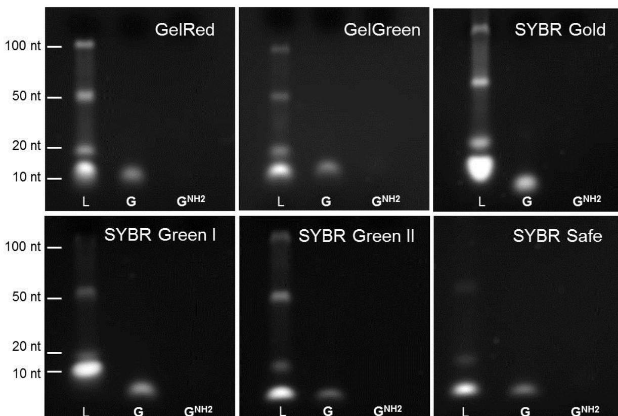
**Figure S6.** Testing of different gel dyes for the visualization of ssONs containing 7-deazaguanosine derivatives instead of natural guanosine. L = DNA ladder, G ssON containing natural guanosine, G<sup>NH2</sup> ssON containing modified 7-deazaguanosine.
