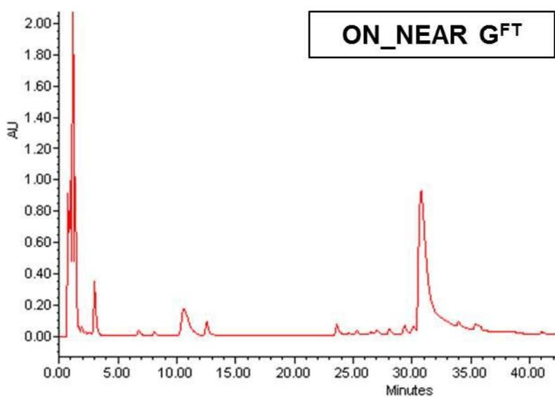
**Figure S4.** HPLC chromatograms of crude NEAR mixtures (preparative reactions). Column XBridge OST C18 2.5  $\mu$ M (4.6  $\times$  50 mm). Mobile phase A: 0.1 M TEAA, B: acetonitrile/0.1M TEAA, 20/80 (v/v). Flow rate: 1 mL/min. Gradient 40 to 80 % B in 53 min.
