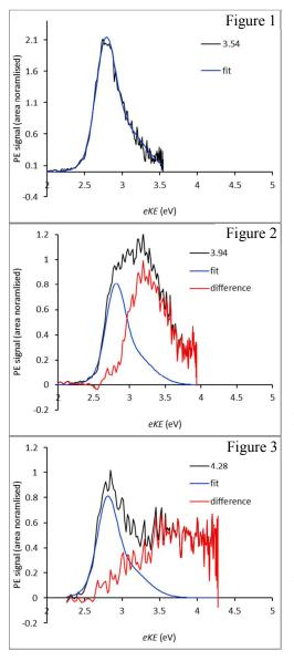
To determine the relative contribution of the  $S_3 \rightarrow D_0$  autodetachment channel compared to all other channels (*i.e.*  $S_3 \rightarrow S_2$  internal conversion), we have fitted the PE spectrum at hv = 3.54 eV to a function (see Figure 1, blue line).
