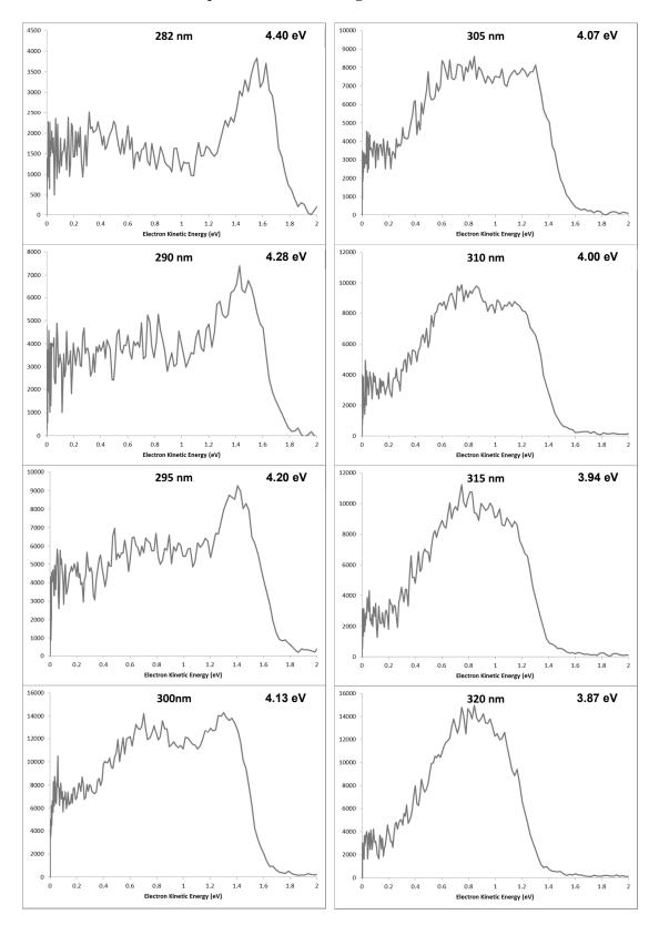
Individual Photoelectron Spectra included in Figure 1e
