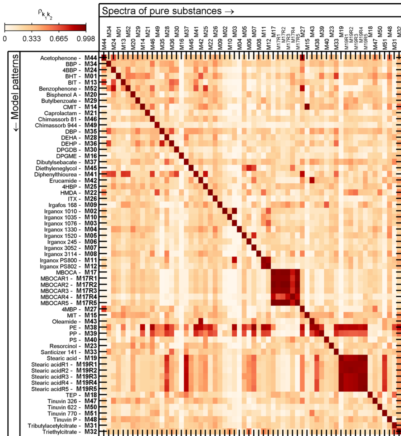
Figure S2. Pairwise correlation coefficients (see Eq. (13) in the main article) between measured spectra of pure substances and spectra encoded as Gaussian lines.
