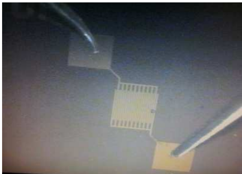
Figure S40. Photograph of interdigitated microelectrodes used for the conductivity measurements.
