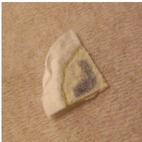
**Figure S2.** The image of a glass fiber separator in the Li cell after exposure to air for several minutes. The previous metallic dark brown part became whitish, indicating the formation of lithium hydroxide (LiOH).
