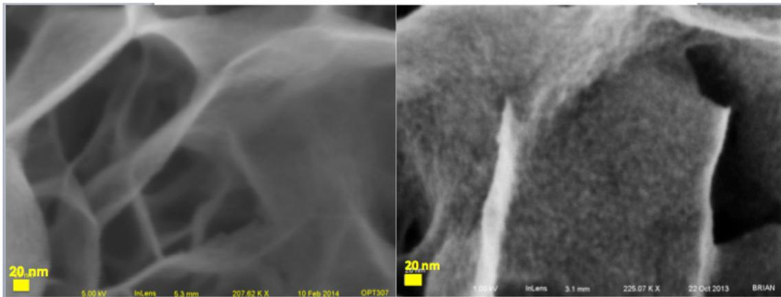
**Figure S4:** SEM of NiO film: before CdSe QD deposition(left) after CdSe deposition(right). Notice the smoothness of the surface of NiO has disappeared upon QD deposition
