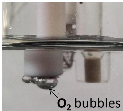
**Figure S7.** Optical photograph showing the generation of oxygen bubbles on Cu<sub>2</sub>S NPs modified GCE.
