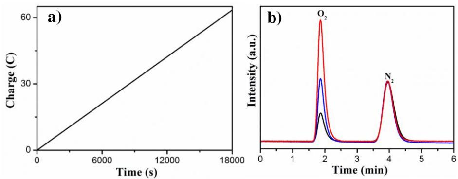
**Figure S10.** (a) Control potential electrolysis of a solution containing 6mM Gly. (b) Normalized gas chromatograms traces from a representative CPE experiment in the presence (red line) and absence (blue line) of 6 mM Gly. Black line shows the air background.
