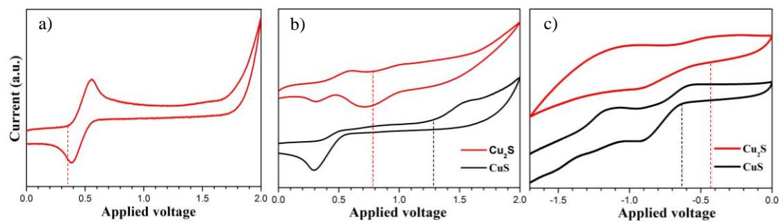
**Figure S2.** (a) The cyclic voltammograms (CV) of the oxidation potential of ferrocene as the internal standard to calibrate the measurements, and (b) oxide and (c) reduction CV of CuS (black line) and Cu<sub>2</sub>S NPs (red line) .
