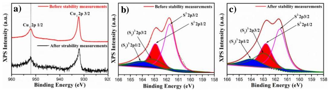
**Figure S9.** XPS spectra of a) Cu 2p, b) and c) S 2p of Cu<sub>2</sub>S NPs before and after the stability measurements.
