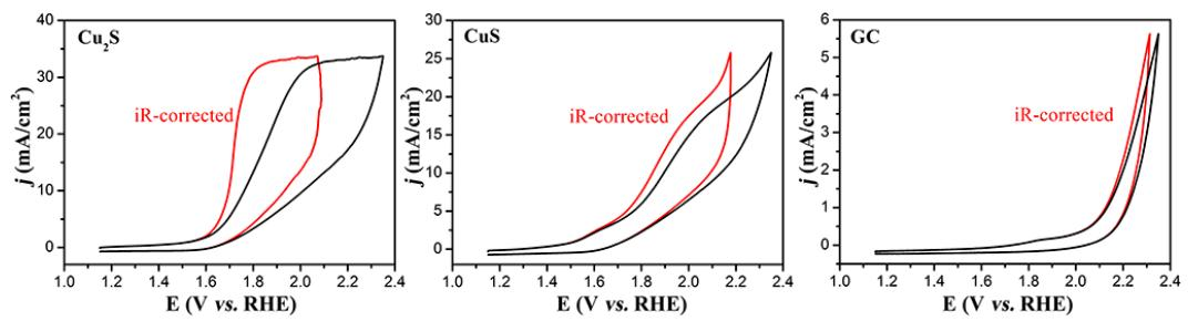
**Figure S6.** iR corrected CV of the Cu<sub>2</sub>S, CuS and GC.
