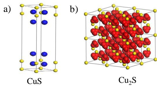
**Figure S4.** The crystal structure of (a) CuS NPs and (b) Cu<sub>2</sub>S NPs.
