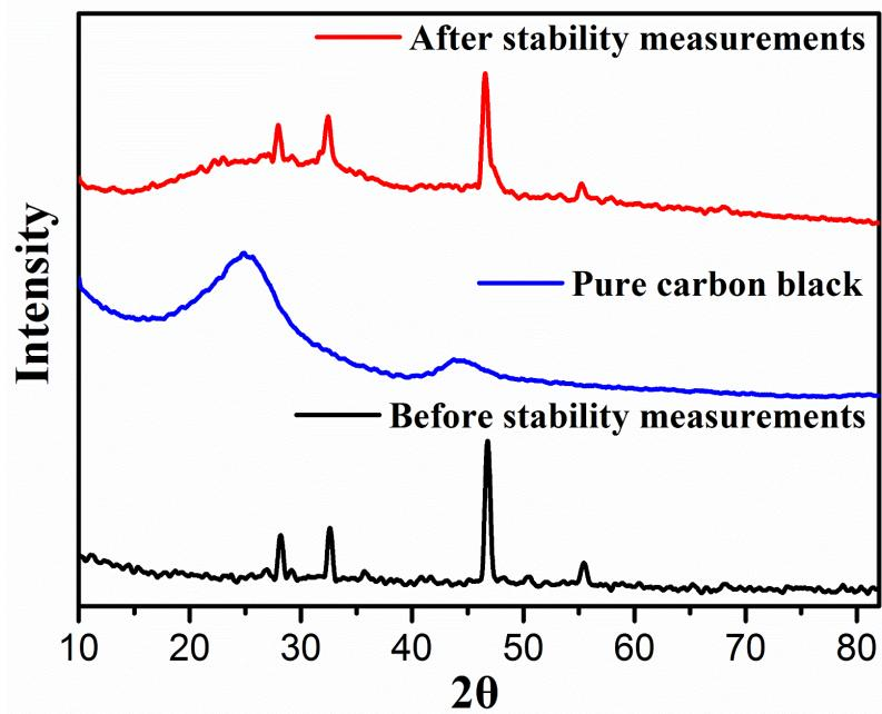
**Figure S8.** XRD pattern of the  $\text{Cu}_2\text{S}$  before and after the stability measurements.
