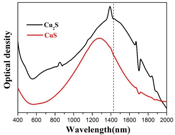
**Figure S1.** The near infrared absorption spectra of the CuS and  $\text{Cu}_2\text{S}$  NPs in chloroform.
