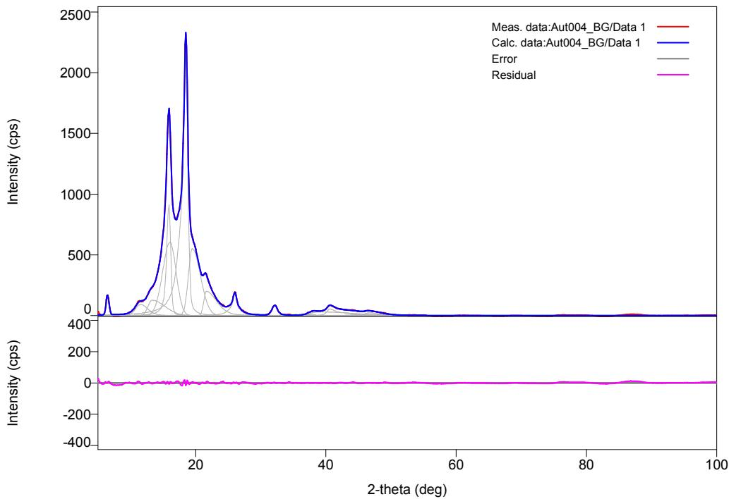
**Figure S32.** WAXRD measurement profile for *syndiotactic* H-poly(DCPD) made from **2** and 50 equiv. of DCPD.
