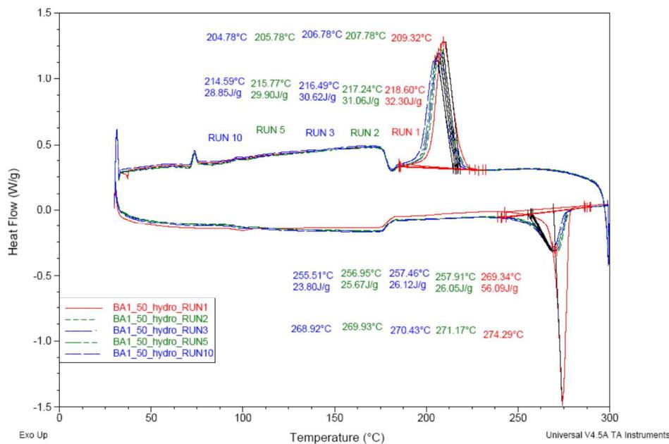
**Figure S23.** DSC thermogram of *syndiotactic* H-poly(DCPD) (50 equiv. DCPD) derived by the action of **2**. 10 heating/cooling cycles. Heating: 10 K/min. Cooling: 20 K/min.
