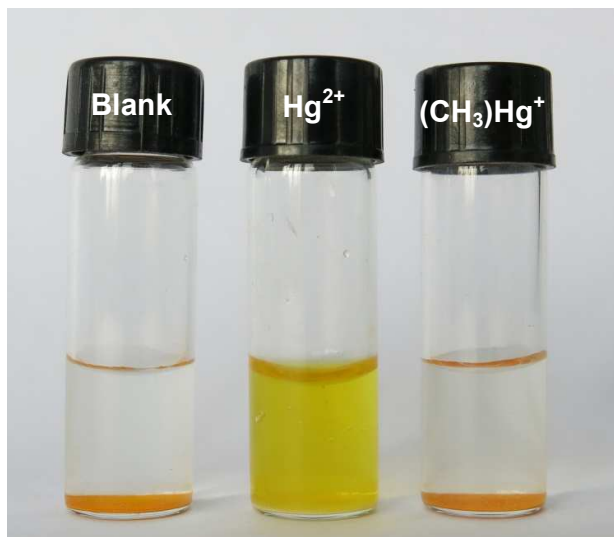
Figure S6. The photos comparing the interactions between RuMOFs and mercury species: inorganic mercury ion ( \text{Hg}^{2+} ) and methylmercury ion ( \text{CH}_3\text{Hg}^+ ). The concentrations of \text{HgCl}_2 and \text{CH}_3\text{HgCl} were all 100 \mu\text{M} . The blank sample: RuMOFs in pure water.
