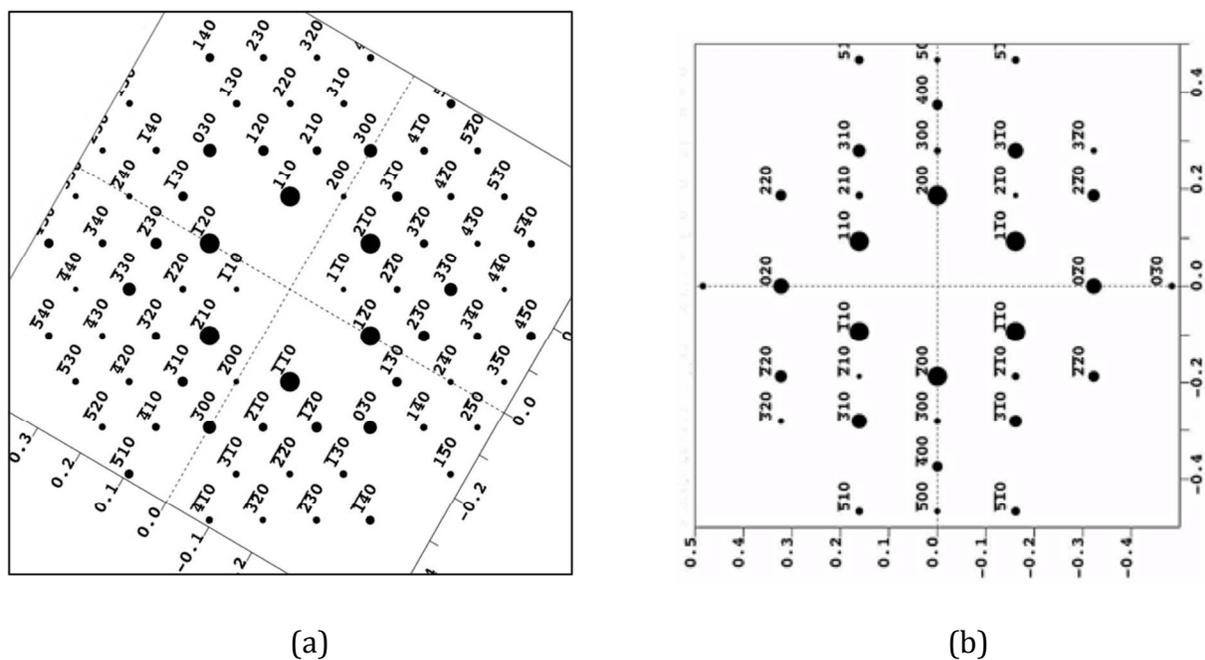
**Figure S1.** Calculated  $hk0$  diffraction patterns of (a) the trigonal, frustrated  $\beta$  phase and (b) the orthorhombic  $\alpha$  crystal phase of PLLA.
