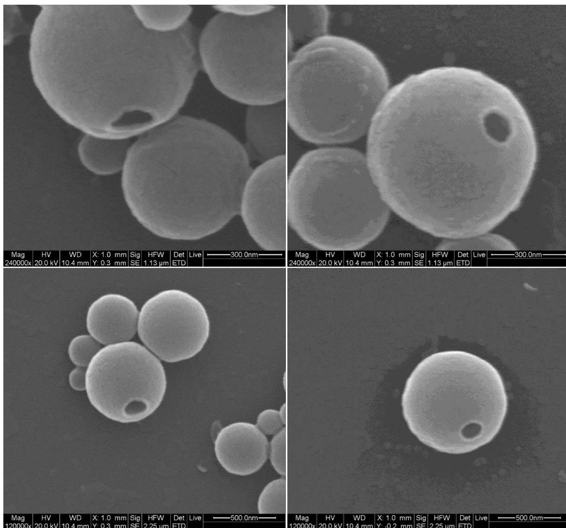
**Figure S6.** More SEM images of nanocapsules with open-mouth holes.
