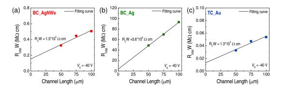
Figure S1 Channel width-normal total resistance as a function of channel length for pentacene OFETs with (a) bottom contact AgNWs, (b) bottom contact Ag, and (c) top-contact Au as source/drain electrodes at  $V_{\rm G}$  = -40 V.
