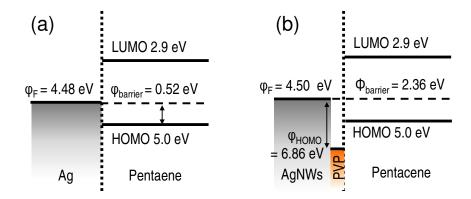
**Figure S2** The band diagram of the interface between metals and pentacene: (a) pentacene/Ag and (b) pentacene/PVP/AgNWs
