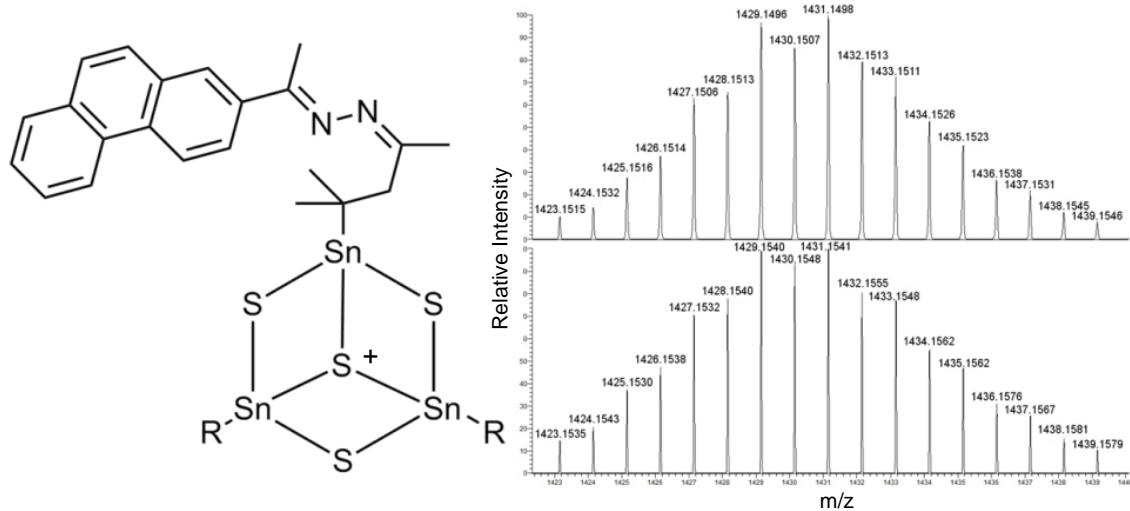
**Figure S5.** Schematic drawing of the cluster cation in **14** (left; R drawn once in detail) along with the high-resolution mass cluster of  $[(C_{22}H_{23}N_2Sn)_3S_4]^+$  as measured by ESI<sup>+</sup> MS (top right) and calculated (bottom right).
