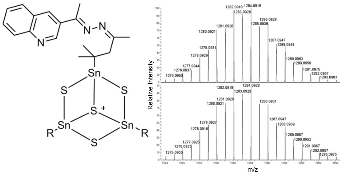
**Figure S2.** Schematic drawing of the cluster cation in **11** (left; R drawn once in detail) along with the high-resolution mass cluster of  $[(\text{C}_{17}\text{H}_{20}\text{N}_3\text{Sn})_3\text{S}_4]^+$  as measured by ESI<sup>+</sup> MS (top right) and calculated (bottom right).
