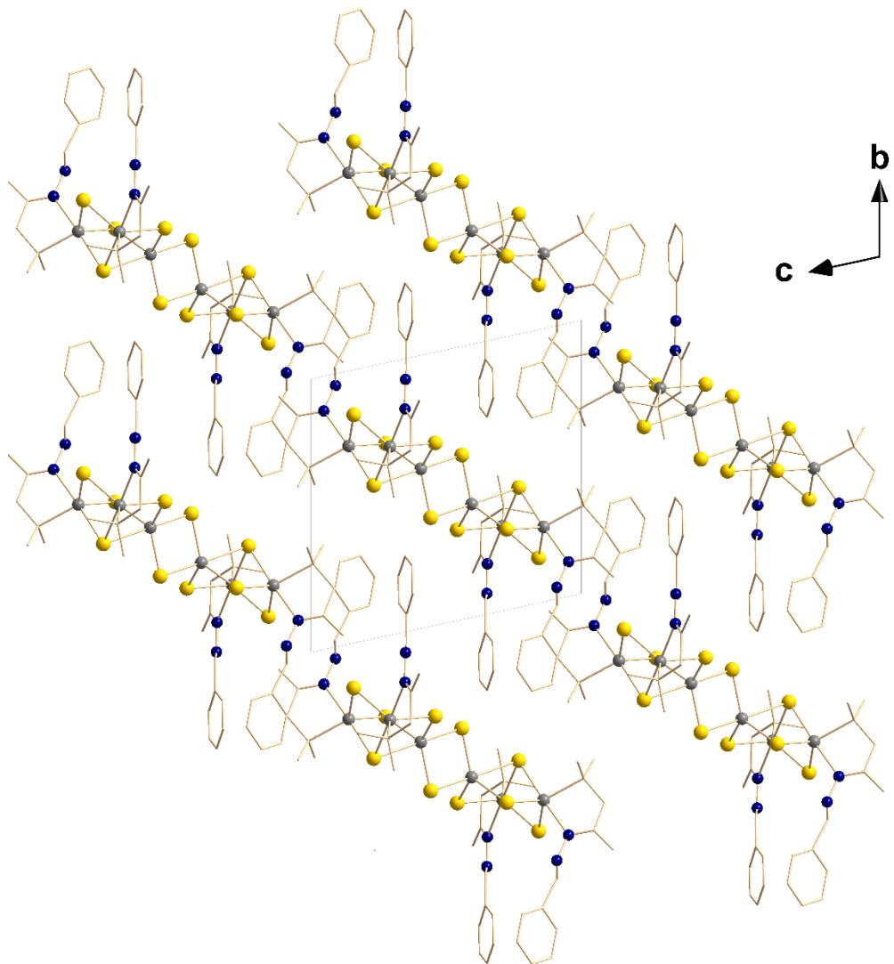
**Figure S7.** Packing of the cluster molecules in compound **6**. Organic moieties are shown as wires, most of the H atoms are omitted for clarity. Yellow spheres: S, grey spheres: Sn, blue spheres: N atoms.
