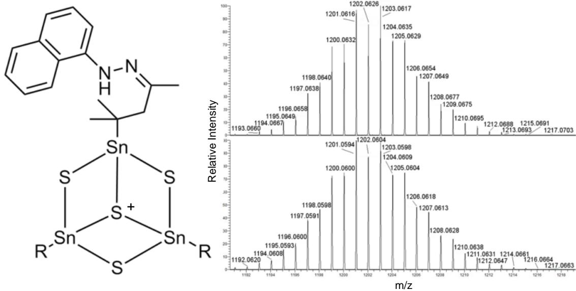
**Figure S6.** Schematic drawing of the cluster cation in **15** (left; R drawn once in detail) along with the high-resolution mass cluster of  $[(C_{16}H_{20}N_2Sn)_3S_4]^+$  as measured by ESI<sup>+</sup> MS (top right) and calculated (bottom right).
