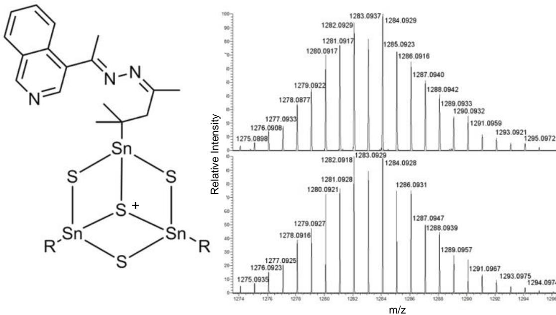
**Figure S3.** Schematic drawing of the cluster cation in **12** (left; R drawn once in detail) along with the high-resolution mass cluster of  $[(\text{C}_{17}\text{H}_{20}\text{N}_3\text{Sn})_3\text{S}_4]^+$  as measured by ESI<sup>+</sup> MS (top right) and calculated (bottom right).
