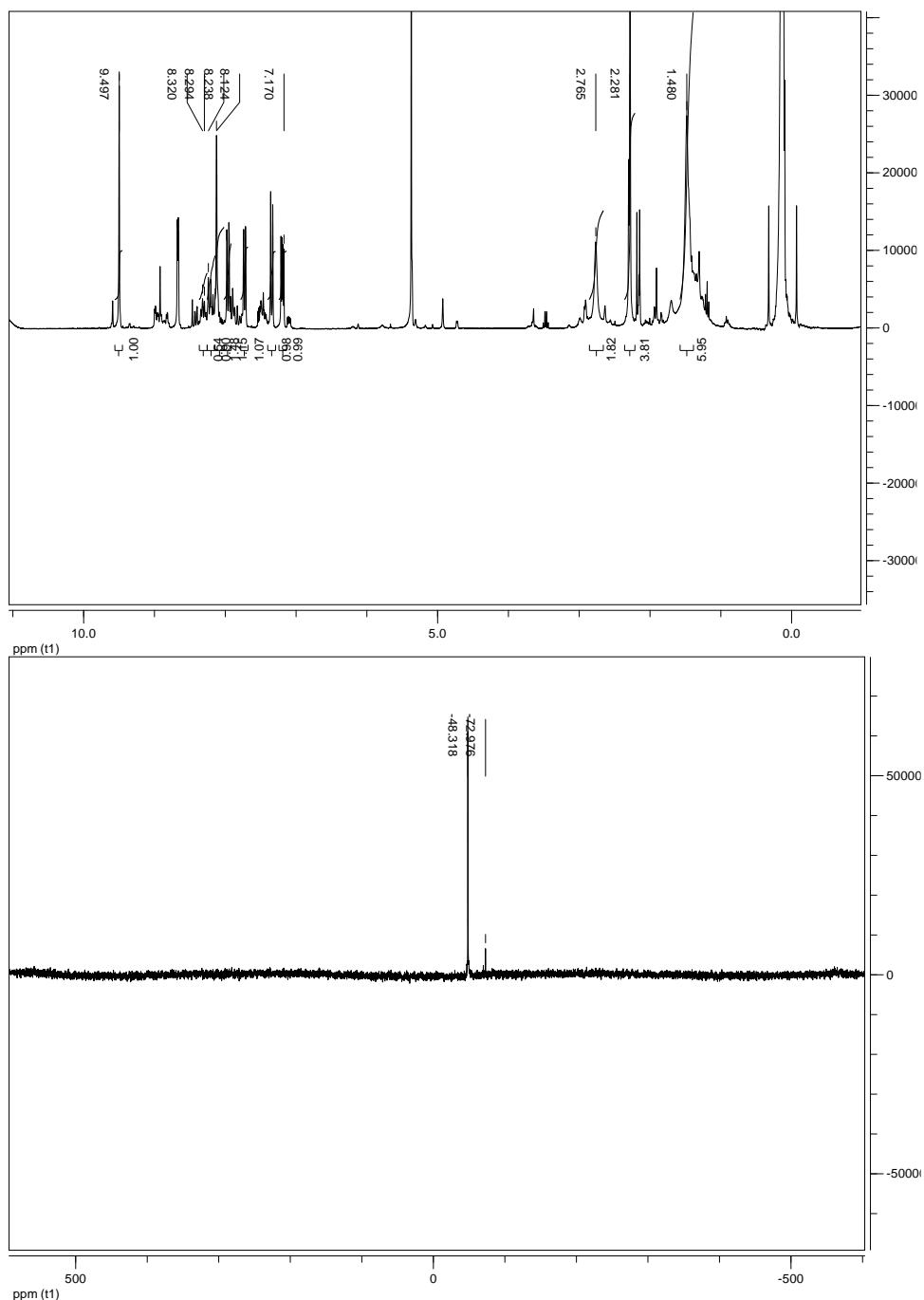
**Figure S8.**  $^1\text{H}$  NMR spectrum (top) and  $^{119}\text{Sn}$  NMR spectrum (bottom) of compound **10**, measured on a saturated solution of single crystals in  $\text{CD}_2\text{Cl}_2$ .
