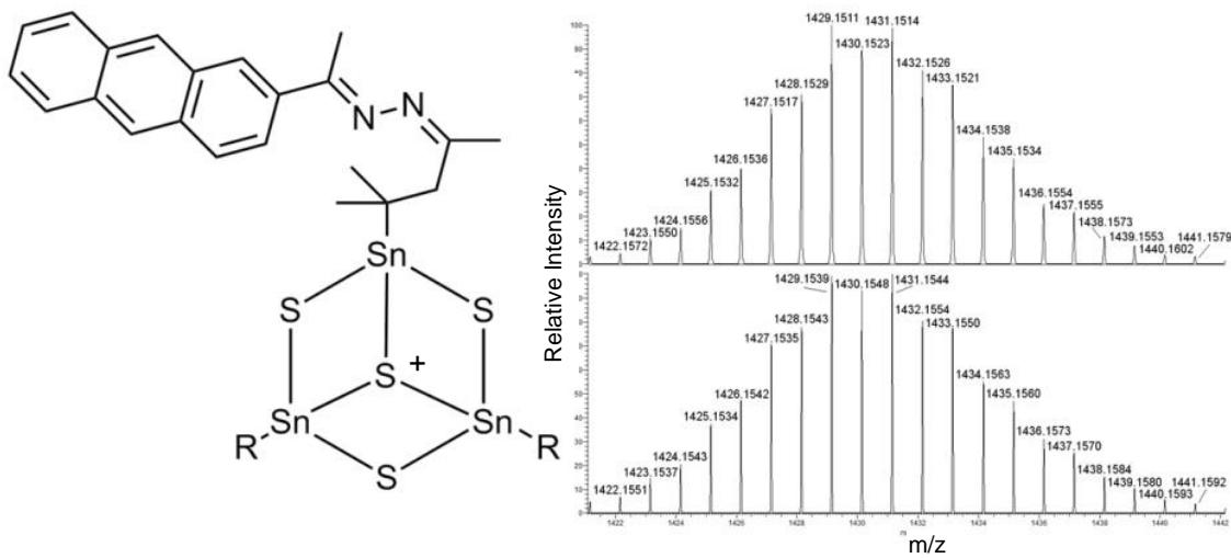
**Figure S4.** Schematic drawing of the cluster cation in **13** (left; R drawn once in detail) along with the high-resolution mass cluster of  $[(C_{22}H_{23}N_2Sn)_3S_4]^+$  as measured by ESI<sup>+</sup> MS (top right) and calculated (bottom right).
