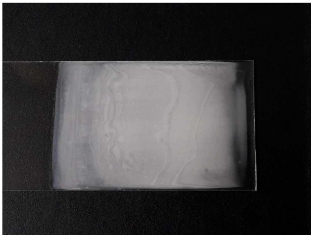
Figure S6. Photo of a 10 wt% ZnO/PS-nanocomposite thin film where the ZnO nanoparticles were coated with oleic acid instead of a polystyrene brush layer. The incompatibility and aggregation of the nanoparticles in the PS (8600 g/ml) matrix are causing pronounced turbidity.
