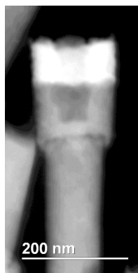
Figure S4. STEM image of a Au nanoring with sacrificial Ni shell segment and Ni base. The effect of pore-widening is evident from the difference in diameter of the Ni rod base and the shell segments.
