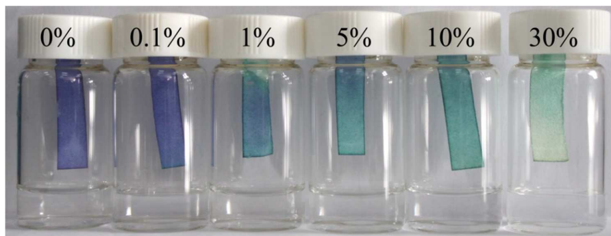
Figure S13. Color changes of CyJ (1.0 mM) coated filter paper after exposure to different concentrations of hydrazine aqueous solution.
