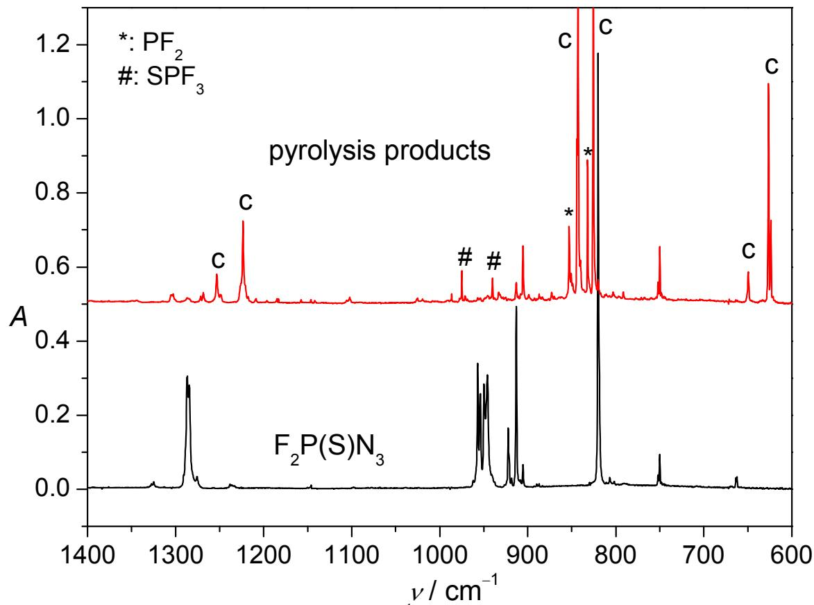
**Figure S4.** Ar-matrix mid-IR spectra ( $1400\text{--}600\text{ cm}^{-1}$ , Transmittance  $T$ ) of  $F_2P(S)N_3$  and its flash vacuum pyrolysis products. The IR bands of  $F_2PNS$  (c) are indicated.
