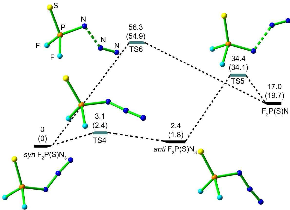
**Figure S6.** Calculated energy profile (kcal mol<sup>-1</sup>) for the decomposition of  $\text{F}_2\text{P}(\text{S})\text{N}_3$  isomers at the CBS-QB3 and B3LYP/6-311+G(3df) (in parentheses) levels.
