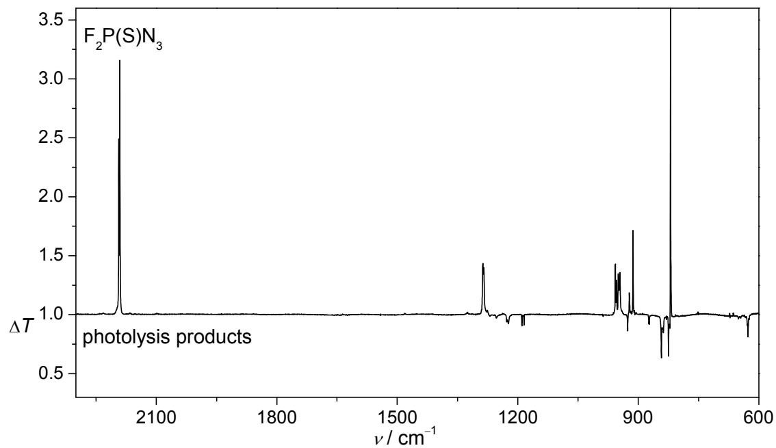
**Figure S1.** Ar-matrix mid-IR difference spectra (2300–600  $\text{cm}^{-1}$ , Transmittance  $T$ ) of the photolysis of  $\text{F}_2\text{P}(\text{S})\text{N}_3$  with ArF laser (193 nm, 1.2 mJ, 20 min).
