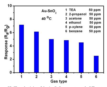
Figure S3. The selectivity of the Au-SnO<sub>2</sub> sensor towards different gases.
