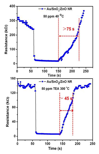
Figure S2. The response-recovery curves of the Au-SnO<sub>2</sub>/ZnO nanorod sensor to 50 ppm TEA working at different temperature.
