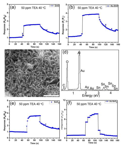
Figure S1. Response and recovery curve of three control sensors, (a) ZnO nanorod sensor; (b) Au-ZnO nanorod sensor; (c) SEM images of Au-SnO<sub>2</sub> nanosheets; (d) EDS spectrum of Au-SnO<sub>2</sub> nanosheets; (e) SnO<sub>2</sub> nanosheet sensor; (f) Au-SnO<sub>2</sub> nanosheet sensor.
