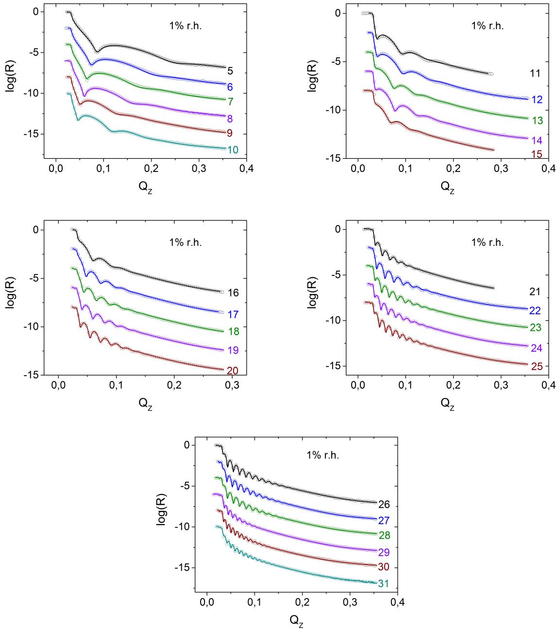
Figure S2: XRR data and fit of PEMs with 5-31 deposited layers measured at 1% r.h.. For better visualization only every 5th data point of measured data is shown in the diagram
