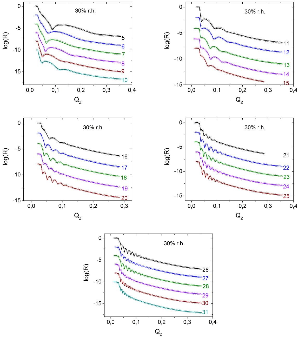
Figure S3: XRR data and fit of PEMs with 5-31 deposited layers measured at 30% r.h.. For better visualization only every 5th data point of measured data is shown in the diagram
