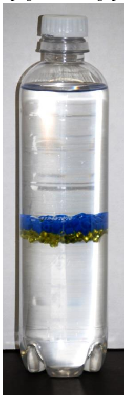
Figure 1: The Dynamic Density Bottle. The liquids and solids layer according to density. From top to bottom: alcohol, blue pieces comprised of LDPE, yellow pieces comprised of PS, 17 % NaCl solution (see also Figure 2, panel at 0 s). Bottle shown is 23 cm high, 20 cm in diameter and holds 500 mL of fluid. See http://www.sparklingice.com/product/blackraspberry for an example of a product with a bottle of these dimensions.
