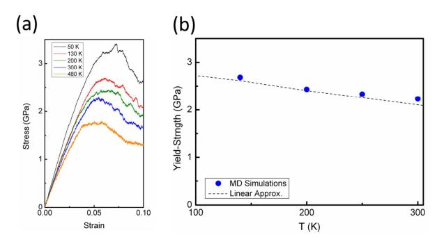
**Fig. S1**| (a) Engineering stress-strain curves for the  $Cu_{60}Zr_{40}$  metallic glass under uniaxial compression test at different temperatures from 50 K to 480 K. (b) Variation of yield strength,  $\sigma_y$ , with temperature at the temperature range of our experiments (130 K-300 K) obtained from molecular dynamics (scattered dots) and the suggested linear approximation to explain the experimental results (dashed-line).
