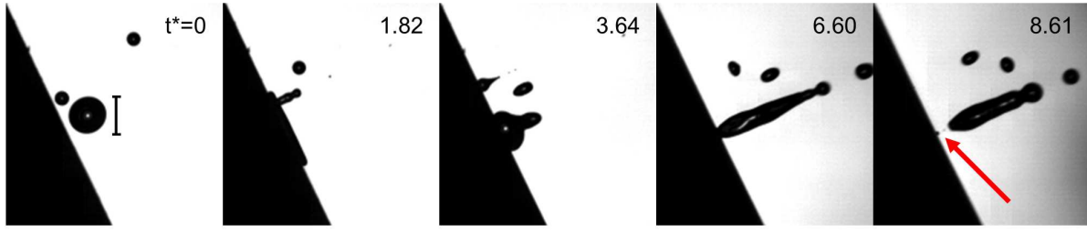
Figure S4. Impact of one large and two small droplets on the t-PTFE surface. Where the two smaller droplets exhibited rebounding behaviour, the arrow at t^*=8.61 indicates the pinned droplet left behind from the larger droplet as a result of partial rebounding. The dimensionless time is given with respect to the large droplet, and the scale bar is 1 mm in length. v_n=1.81 m/s, v_t=0.10 m/s, D=0.95, 0.35, 0.33 mm.
