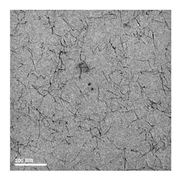
**Figure S1.** Transmission electron micrograph depicting the stable dispersion of  $TiO_2$  NRs in PS matrix (M = 650 kDa,  $\phi_{NR}$  = 0.01) after thermal annealing at 190 ° C for 6hrs.
