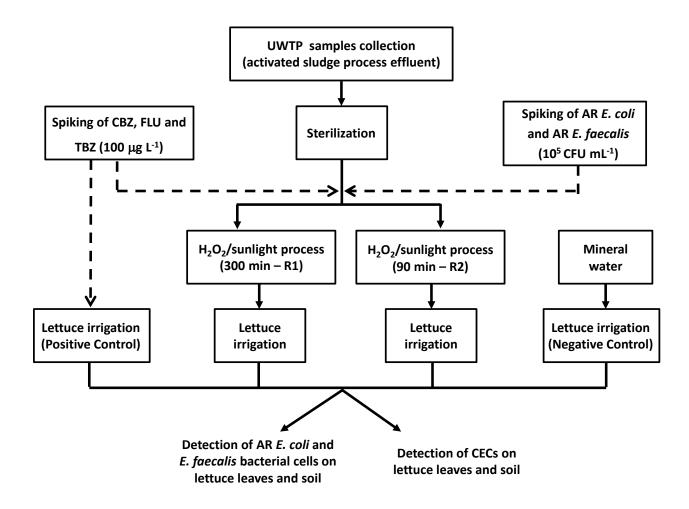
**Figure S1.** Schematic view of experimental design. Acronyms: Carbamazepine (CBZ), flumequine (FLU), thiabendazole (TBZ), antibiotic resistant (AR), urban wastewater treatment plant (UWTP).
