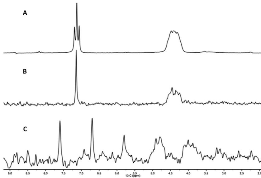
**Figure S1.** The  $^{13}\text{C}$  NMR spectrum of complex **3c** recorded in  $\text{C}_6\text{D}_6$  in the region corresponding to the metal-bound methyl groups. (A) Sample enriched in  $^{13}\text{C}$ . (B) Sample with natural abundance. (C) Proton-coupled spectrum.
