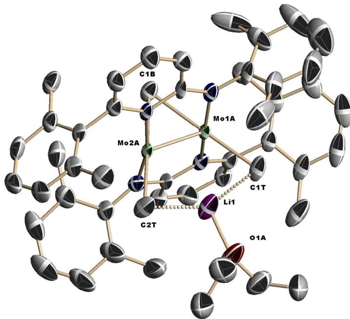
**Figure S4.** The solid-state molecular structure of **3b**, with thermal ellipsoids set at 30% probability. All hydrogen atoms are omitted for clarity. Selected bond lengths ( $\text{\AA}$ ): Mo(1)–Mo(2), 2.084(7); Mo(1A)–N(1), 2.111(6); Mo(1A)–N(3), 2.176(6); Mo(1A)–C(1T), 2.273(8); Mo(2A)–N(4), 2.117(7); Mo(2A)–N(2), 2.191(6); Mo(2)–C(2T), 2.251(7); Mo(2A)–C(1B), 2.411(7); C(2T)–Li(1), 2.162(6); C(1T)–Li(1), 2.160(5); O(1A)–Li(1) 1.954(2).
