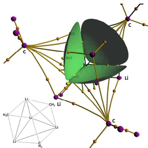
Figure S7. Molecular graph of  $\text{Me}_4\text{Li}_4$  showing bcp's as orange balls and interbasin surfaces for one of the lithium atoms.
