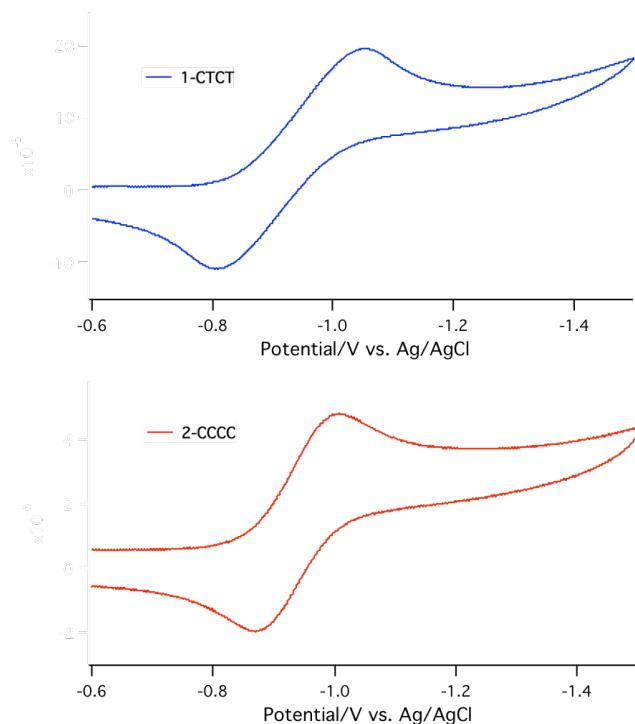
**Figure S18.** Cyclic voltammograms for **1-CTCT** (blue) and **2-CCCC** (red).
