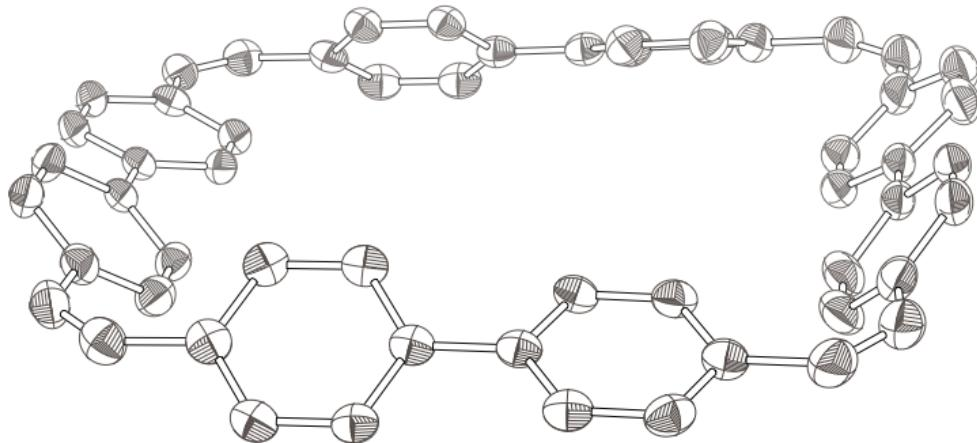
**Figure S12.** Molecular structure of 2-CCCC. Hydrogen atoms are omitted for clarity.
