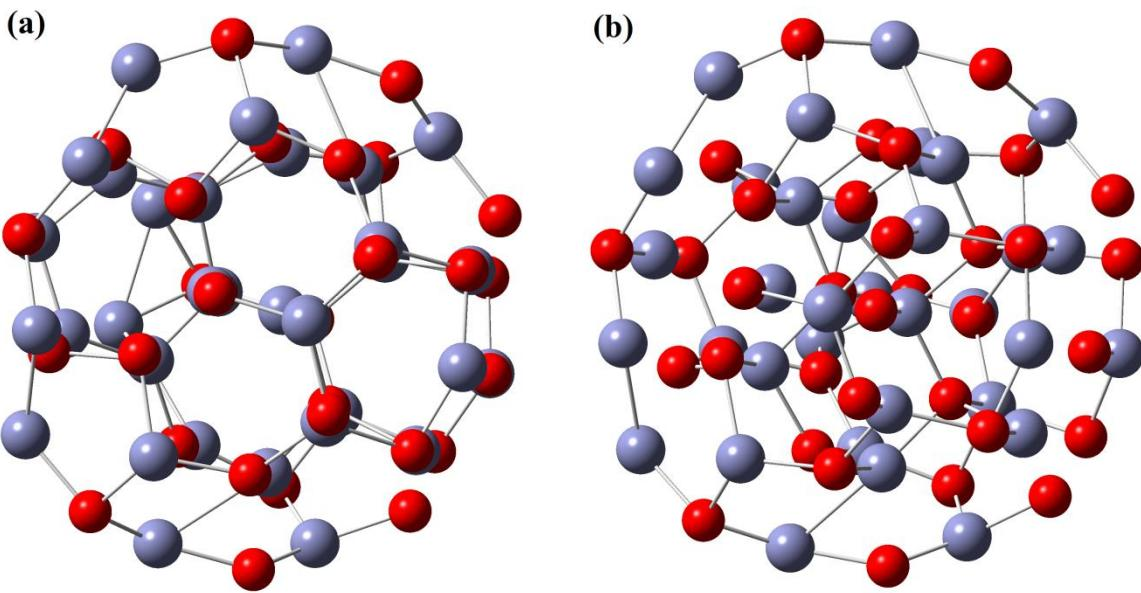
**Figure S3.** Top and side view of the modelled structure of  $(\text{ZnO})_{34}$  cluster without optimization represented by (a) and (b), respectively. Colour code: blue for Zinc atoms and red for Oxygen atoms.
