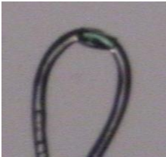
Figure S8. (a) Crystal shape of 3 mounted on thin polyimide films (MiTeGen MicroMounts). (b) Crystal shape calculated by Rigaku RAPID-II.
