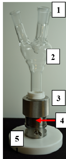
Figure S1: Self-made electrolysis vessel for the surface modification of Ag-NWs.
