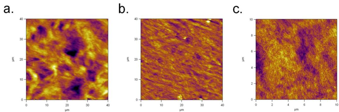
**Figure S6.** AFM images of the self-templated Control-PA structures. **a**, pulled at 30  $\mu\text{m}/\text{min}$  from 10 mg/mL of Control-PA solution. **b**, pulled at 50  $\mu\text{m}/\text{min}$  from 10 mg/mL of Control-PA solution. **c**, pulled at 30  $\mu\text{m}/\text{min}$  from 5 mg/mL of Control-PA solution.
