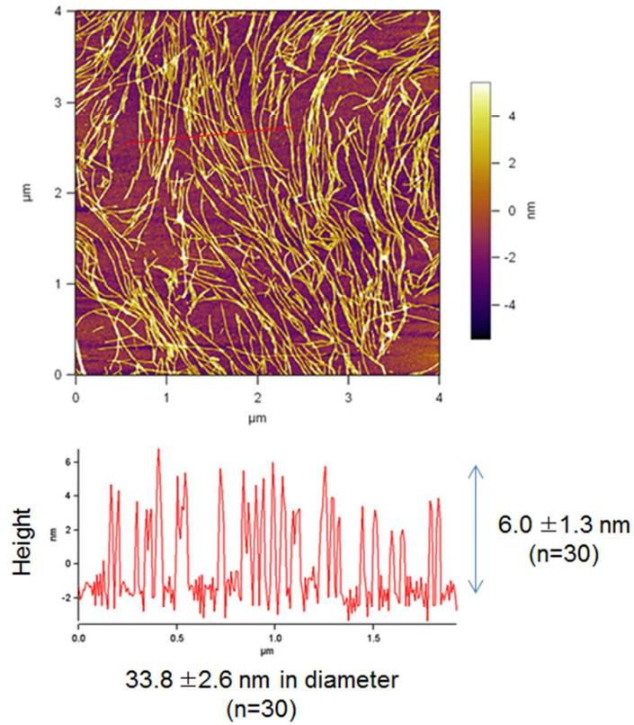
**Figure S2.** AFM image and cross-sectional profile of CLPA nanofibers. The nanofibers were formed from a drop-cast CLPA solution ( $10 \mu\text{g/mL}$ ).
