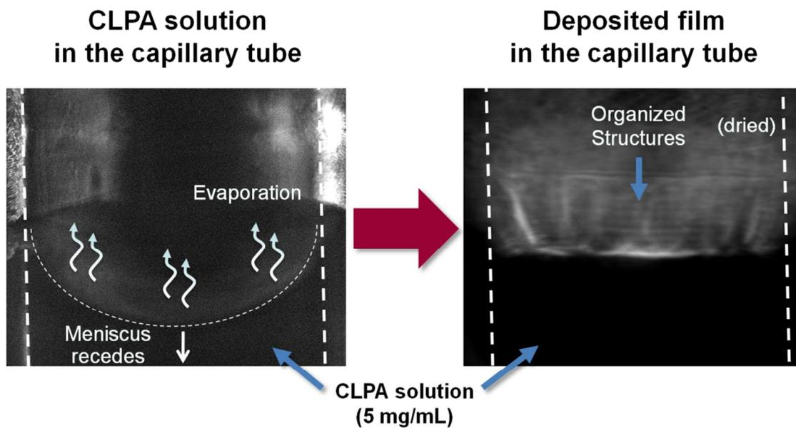
**Figure S3.** Polarized optical microscope image of the meniscus area of CLPA (5 mg/mL) filled in the capillary tube. As the meniscus receded the organized structures were deposited on the wall of the capillary tube.
