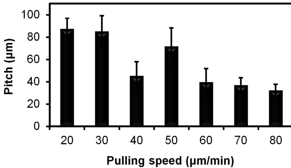
**Figure S5.** Structural periodicity in twisted plywood-like phase structures (1 mg/mL) depends on pulling speed.
