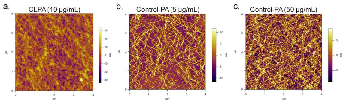
**Figure S1.** AFM images of drop cast CLPA and Control-PA on Si substrates. **a-c**, 10 µL of solution was dropped on a Si wafer and dried at room temperature.
