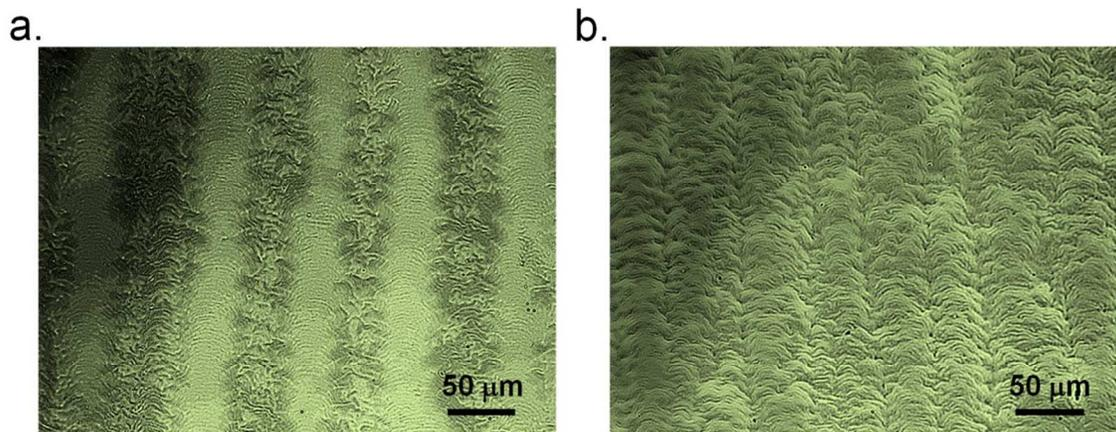
**Figure S4.** Optical microscope images of twisted plywood-like structures created by pulling a substrate at: 30  $\mu\text{m}/\text{min}$  (a); and 70  $\mu\text{m}/\text{min}$  (b) from 1 mg/mL of CLPA solution.
