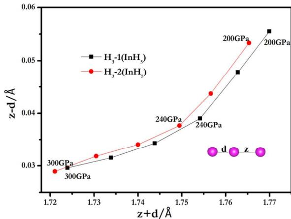
**Figure S2** The difference between the  $z$  and  $d$  distances in an  $\text{H}^-\cdots\text{H}_2$  fragment is plotted vs their sum for  $H_3$  units in  $\text{InH}_5$  at different pressures.
