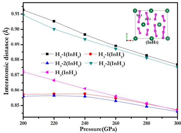
**Figure S1** The pressure dependence of the H-H distance in  $H_3$  units in  $\text{InH}_3\text{-R-3}$  and  $\text{InH}_5\text{-P-1}$  structures. And  $H_3\text{-1}$  and  $H_3\text{-2}$  represent the two different types of  $H_3$  in  $\text{InH}_5\text{-P-1}$  phase.
