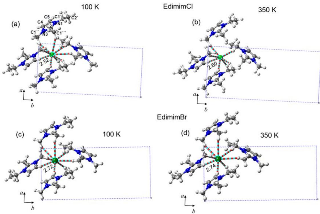
**Figure S4.** Hydrogen-bonding network in Edimid[Cl] at (a) 100 K and (b) 350 K and Edimid[Br] at (c) 100 K and (d) 350 K (H—Cl and H—Br contact up to 3.10 and 3.20 Å are marked with green and red stripes). The shorter hydrogen-bonding distance is displayed.
