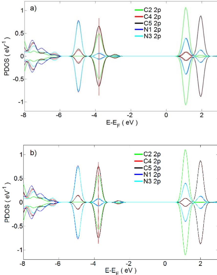
**Figure S5 | PDOS of in the imidazolium ring for (a) Edimid[Cl] and (b) Edimid[Br] at 0 K. Dashed line shows the state with energy of -3.79 eV (a) and -3.81 eV (b) form below the Fermi energy, where the  $\pi^+-\pi^+$  interactions are detected.**
