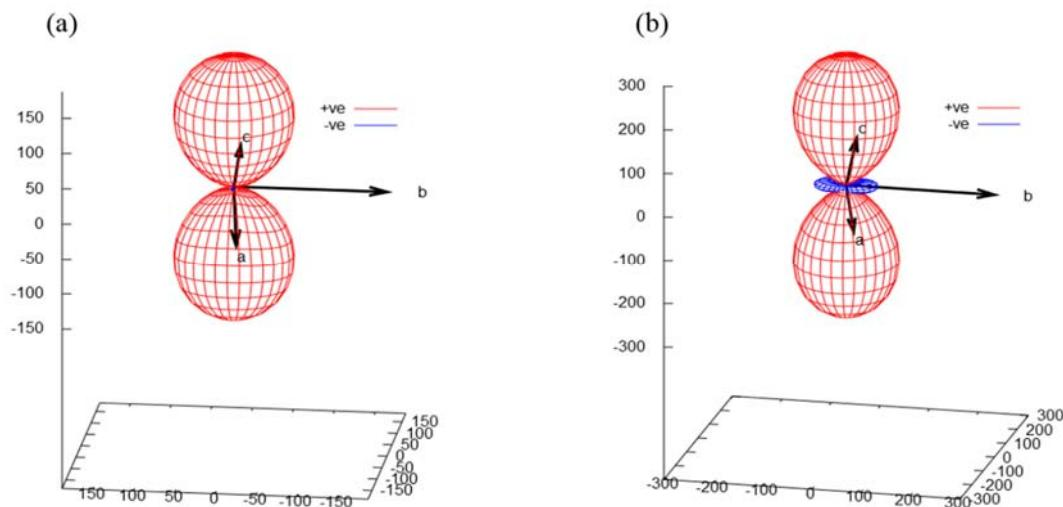
**Figure S3.** The thermal expansion indicatrices (red positive; blue negative) of (a) Edimidim[Cl] and (b) Edimidim[Br] related to the crystallographic axes (black).
