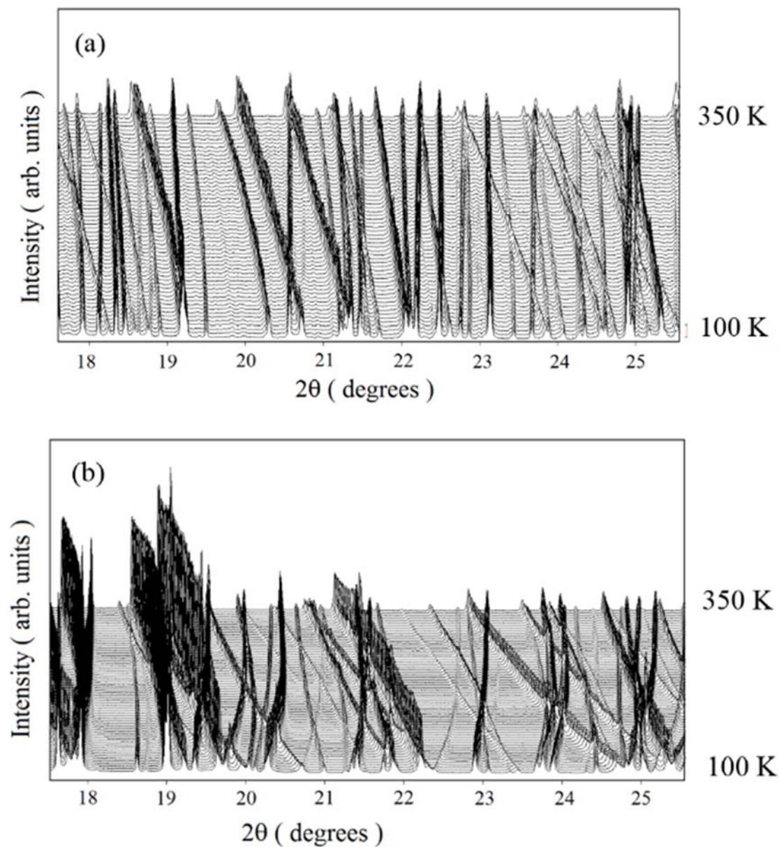
**Figure S2. Thermal evolution of Synchrotron powder data collection between 100 and 350 K from 17.5 to 26 ° for (a) chloride and (b) bromide salts.**
