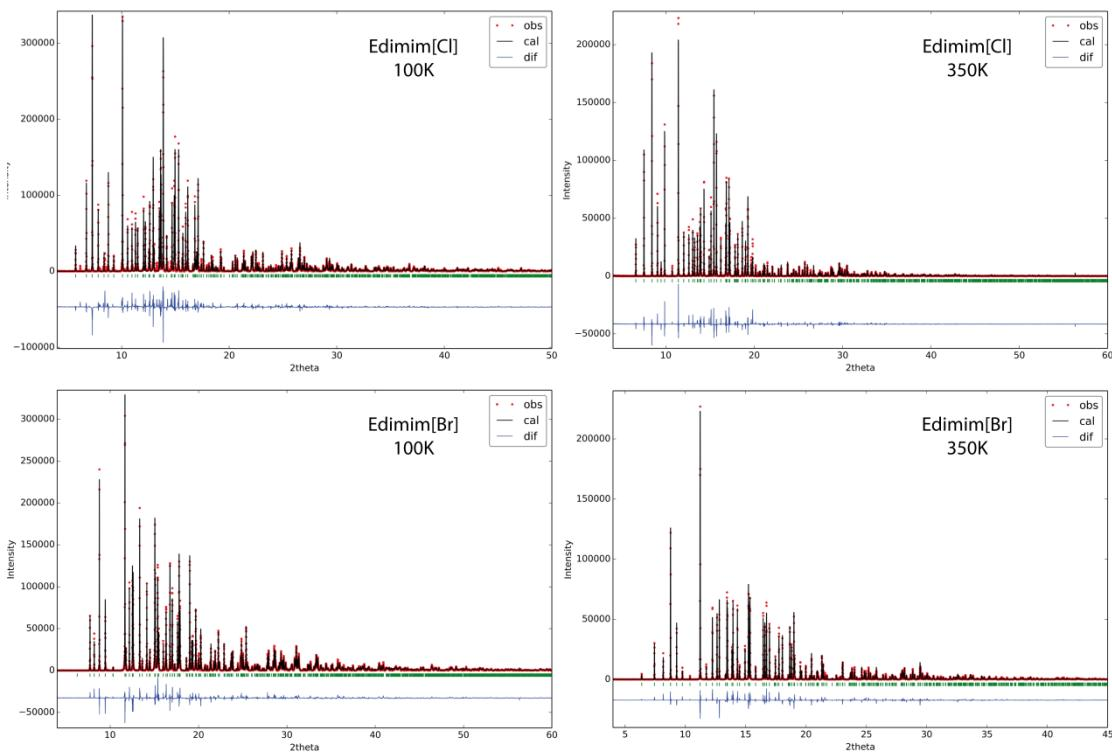
**Figure S1.** Observed (red points) and calculated (blue solid line) powder diffraction patterns for Edimidim[Cl] at (a) 100 K and (b) 350 K, and Edimidim[Br] at (c) 100 K and (d) 350 K. Positions of the Bragg reflections are represented by vertical bars. The observed-calculated difference patterns are depicted at the bottom of each figure.
