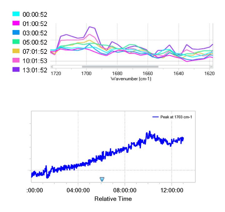
Potassium hydroxide (0.15 mmol) was weighed into a 25 mL Schlenk tube. Then benzyl alcohol (3 mL) was added. The IR probe was inserted through an adapter into the Schlenk tube. Then air balloon was connected to the branch of Schlenk tube. The reaction vessel was kept in 130  $^{\circ}$ C and operando IR spectra was recorded over the course of the reaction.
