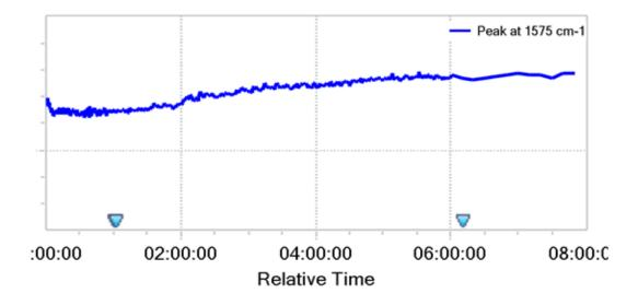
*N*-benzylidene-4-methylbenzenesulfonamide (2 mmol) and KOH (0.1 mmol) were weighed into a 25 mL Schlenk tube. After dried *in vacuo* for 15 min, benzyl alcohol (2 mL) was added. The IR probe was inserted into the Schlenk tube through an adapter under argon flow. The reaction vessel was kept in 130  $^{\circ}$ C and operando IR spectra was recorded over the course of the reaction (*Imine vanished soon after heating up to 130 °C*).
