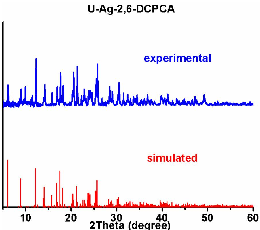
**Figure S3.** Powder x-ray diffraction of U-Ag-2,6-DCPCA. The experimental spectrum (upper diagram) is in good accordance with the simulated spectra from single crystal data (lower diagram).
