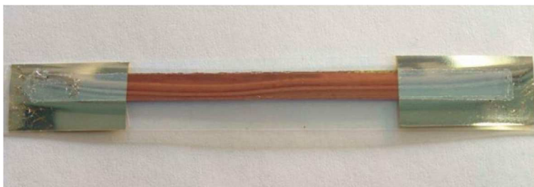
Figure S11. Picture of a sintered Cu strip with evaporated Ag contact pads used for long-term stability measurements and bending tests.
