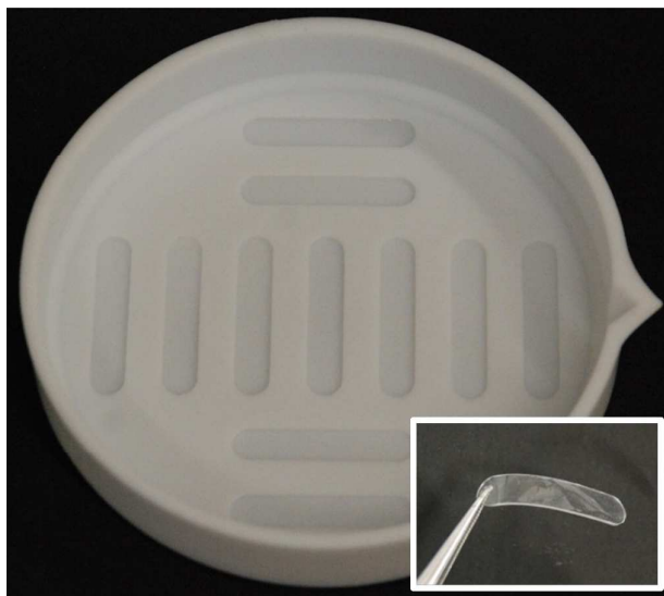
Figure S6. Pictures of a poly(tetrafluoro ethylene) (PTFE) mold with sample cavities (30 mm x 5 mm x 0.4 mm) (large picture) and a polymer sample made with this mold (inset).
