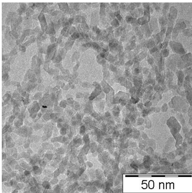
**Figure S1.** TEM image of SnO<sub>2</sub> nanoparticles.
