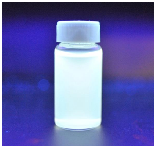
Figure S2. Photograph demonstrating fluorescence emitted by a dilute aqueous solution of GQDs (0.125 mg/mL) under UV light
