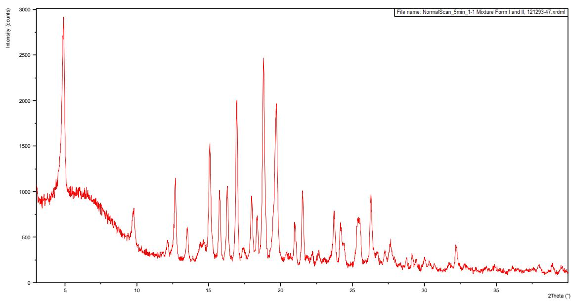
Figure S1: X-ray diffraction pattern of 1:1 w/w mixture of Form 1 and Form 2.
