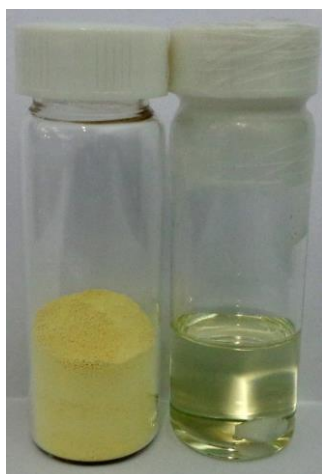
Figure S1. Photo of bulk GPPCN (left) and GPPCN/H 2 SO 4 solution (50 mg/mL, right).
