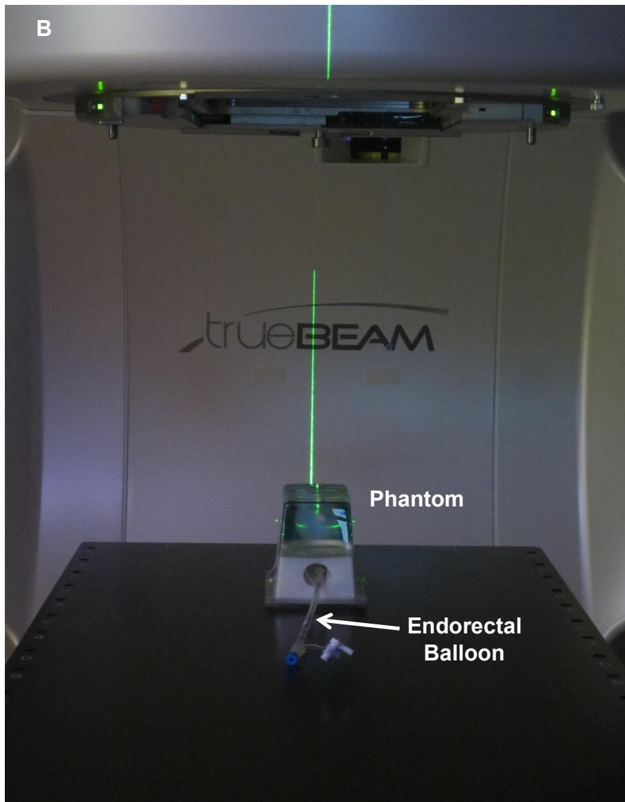
**Figure S12.** Digital images showing the anthropomorphic prostate phantom irradiation set up on the linear accelerator at the Banner-MD Anderson Cancer Center in Gilbert, AZ. (A) Top view and (B) front-on / side view.
