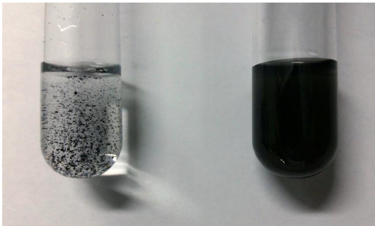
**Figure S1.** Comparison between undispersed SWNTs (left) and well-dispersed SWNTs using B-ssDNA and BSA.
