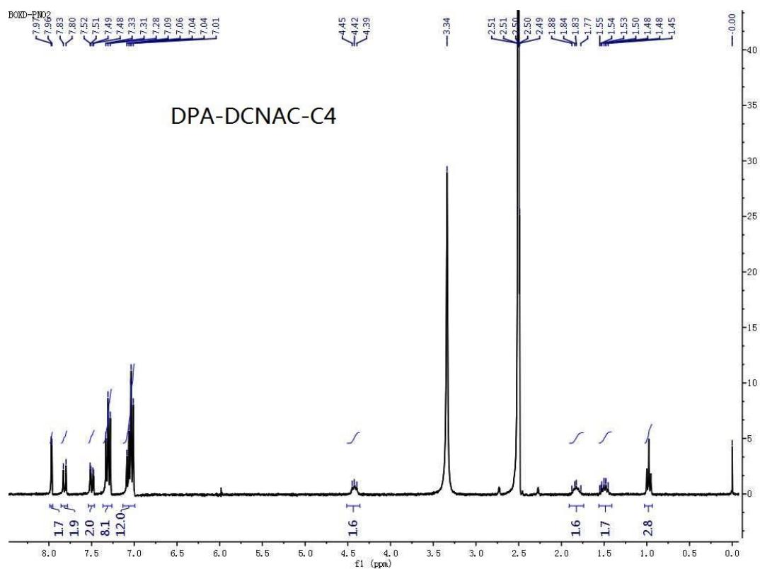
**Figure S13.**  $^1\text{H}$  NMR of DPA-DCNAC-C4 in  $\text{DMSO}-d_6$ .
