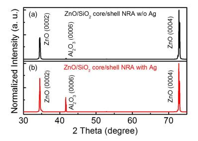
**Figure S2.** XRD patterns of the  $ZnO/SiO_2$  core/shell NRAs without (a) and with (b) Ag NPs decoration, respectively; the thickness of SiO<sub>2</sub> shell is 12 nm.
