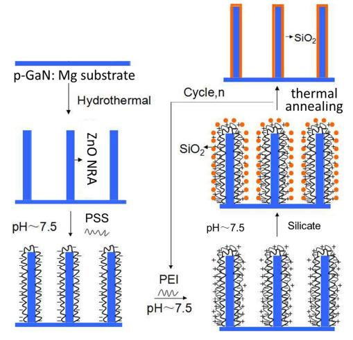
Figure S1. Schematic flow charts for the preparation of ZnO/SiO<sub>2</sub> core/shell NRAs.
