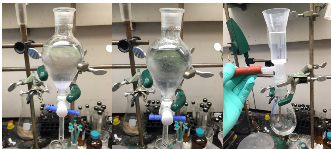
(Left) After 1M HCl (aq) wash. (Center) After brine wash. (Right) Filtering the drying agent.
