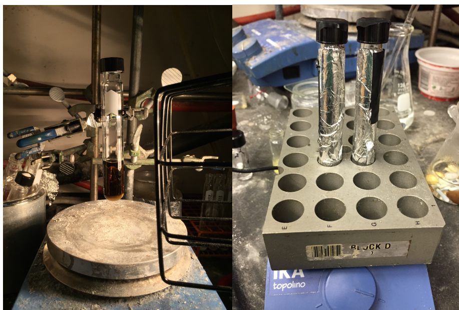
Left: reaction of 1a with 2 in the presence of di- t Bubipy irradiated with a 300 W lamp. Right: reaction of 1a with 2 in the presence of di- t Bubipy in the dark.
