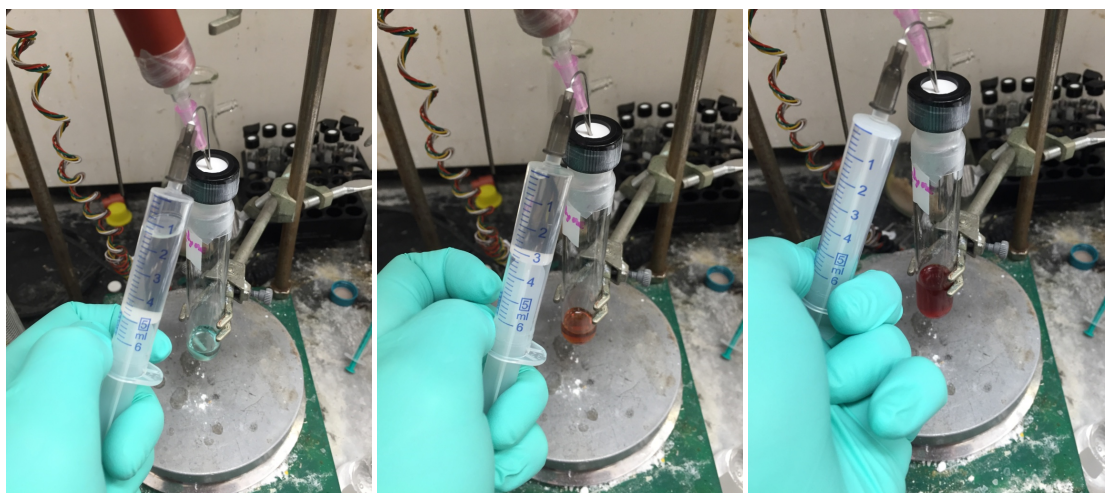
(Left) Prior to addition of 3-OMePhZnCl•LiCl. (Center) A red/brown color is immediately evident. (Right) Completed addition of 3-OMePhZnCl•LiCl solution.
