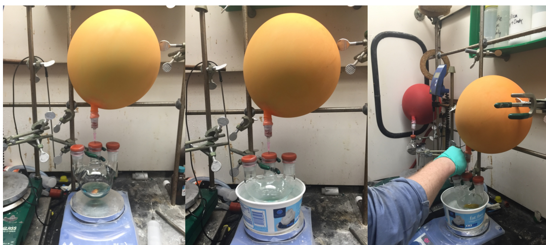
(Left) Reaction flask after addition of redox-active ester. (Center) Reaction flask placed in water bath. (Right) Addition of \text{PhZnCl} \cdot \text{LiCl} in THF.
