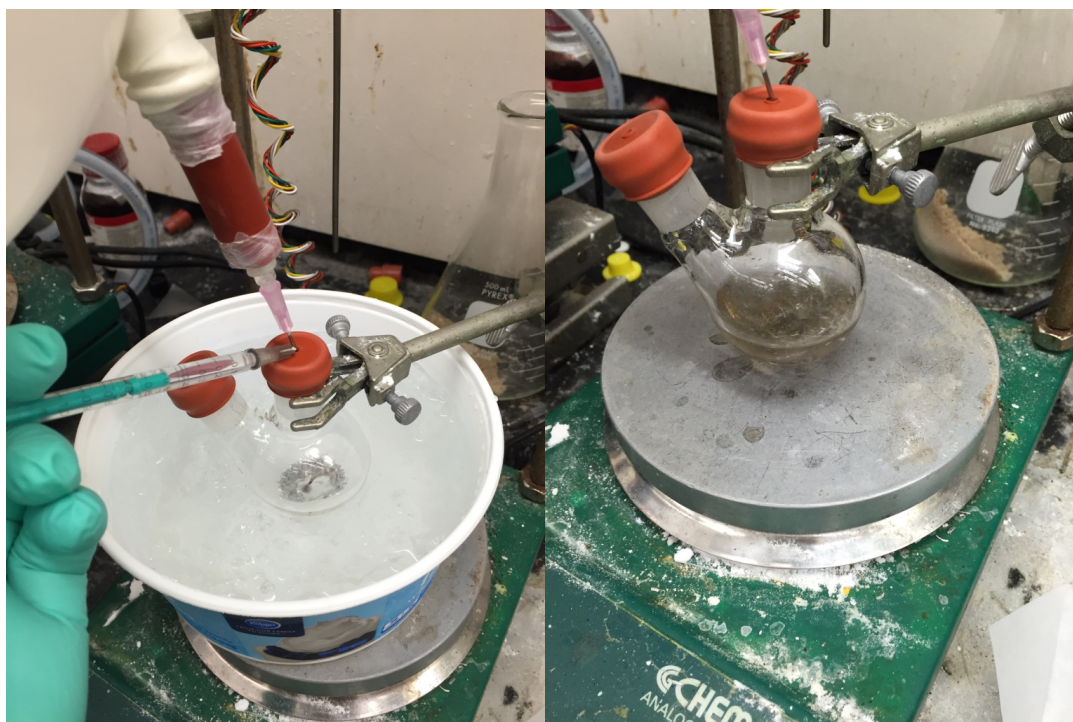
(Left) Addition of 3-bromoanisole at 0 °C (ice/water bath). (Right) Color change of solution after 30 minutes.
