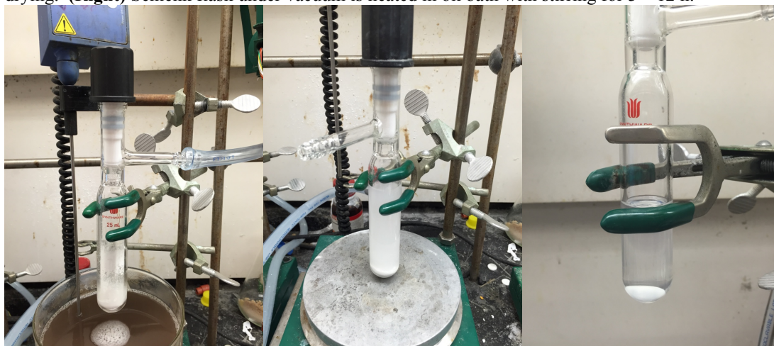
(Left) The Schlenk flask is removed from the oil bath and allowed to cool to rt. (Center) After 10 min of vigorous stirring. To fully dissolve all solids requires longer stirring times, but use of this solution at this stage in preparation of arylzinc does not result in subpar reaction performance. (Right) \text{ZnCl}_2 (1M in THF) after 12 h of stirring.
