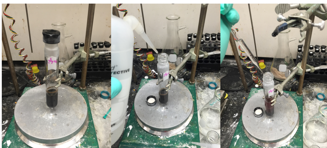
(Left) Reaction with NiCl 2 •glyme after 12 hr. A black color is often observed but is not imperative to the success of the reaction. (Center) Dilution with Et 2 O. (Right) Slow addition of 1M HCl (aq).
