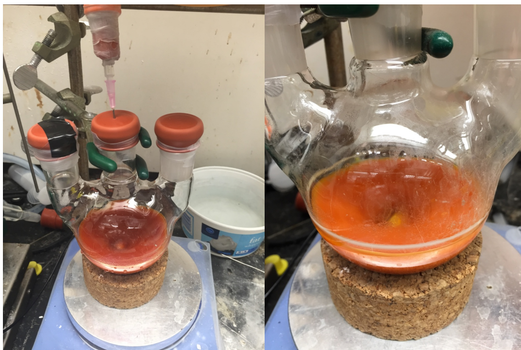
(Left) Removal of flask from water bath to stir overnight. (Right) Reaction mixture after 16 h.
