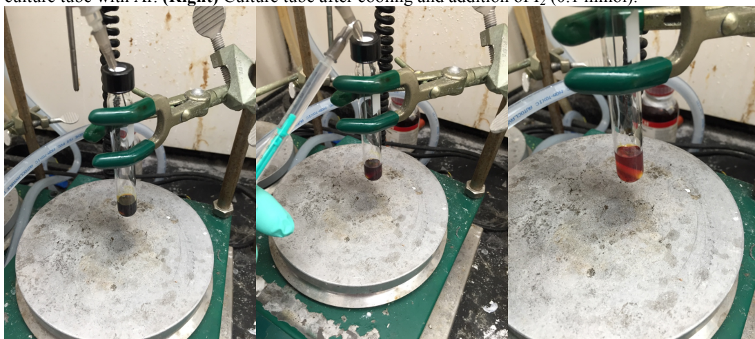
(Left) After addition of THF (1.0 mL) to I_2 and LiCl. (Center) Beginning of the titration. (Right) Progression of the titration.
