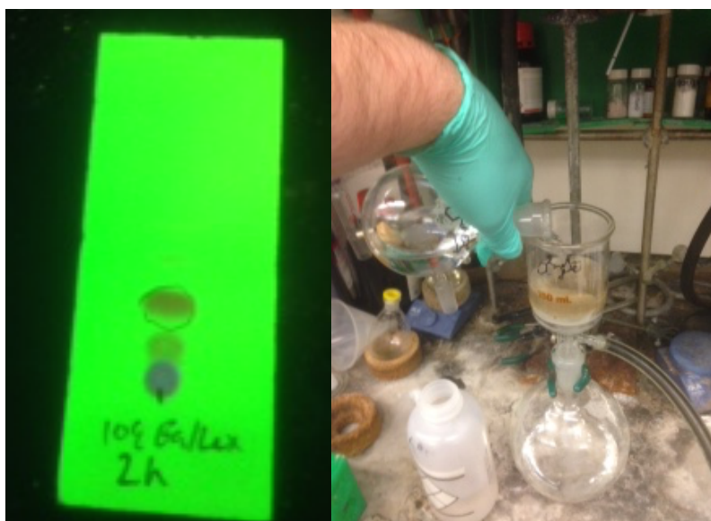
(Left) TLC of reaction mixture after 2 h (9:1 hexanes:EtOAc). (Right) The reaction was passed over a pad of silica (rinsed with EtOAc).
