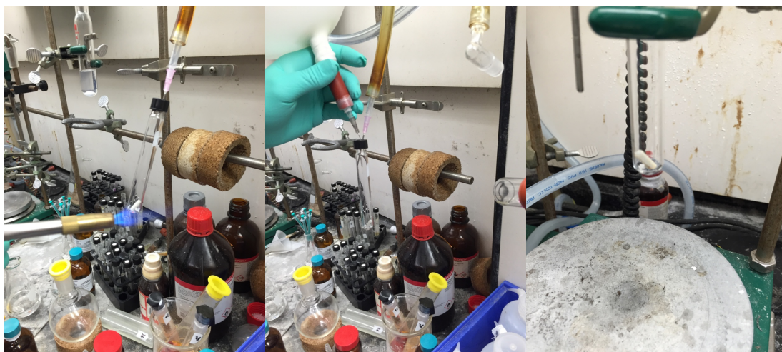
(Left) Flame-drying a culture tube equipped with stir bar and LiCl (0.5 mmol). (Center) Backfilling culture tube with Ar. (Right) Culture tube after cooling and addition of I_2 (0.1 mmol).
