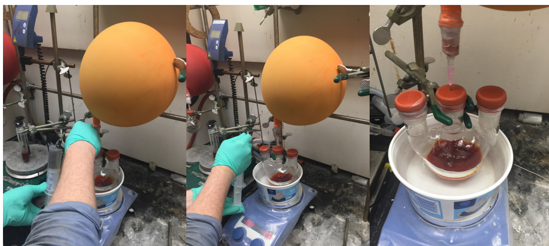
(Left and Center) Progression of addition of \text{PhZnCl} \cdot \text{LiCl} in THF (Right) After addition of \text{PhZnCl} \cdot \text{LiCl} in THF.
