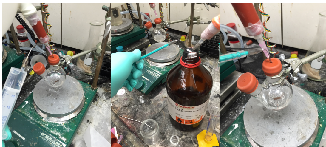
(Left) Addition of THF to Mg and LiCl. (Center and Right) Addition of DIBAL-H (1.0 M in THF) via syringe.
