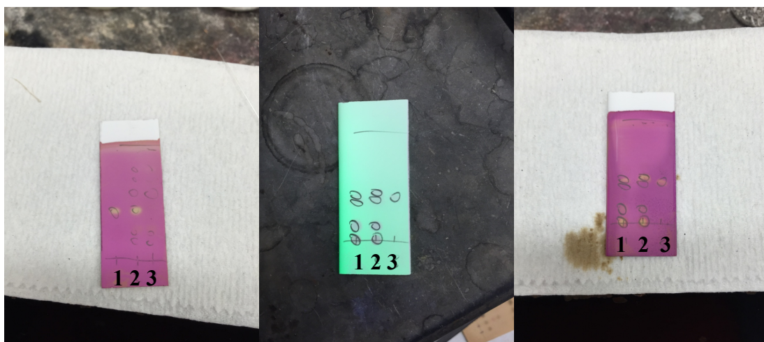
(Left) TLC (4:1 hexanes:EtOAc). Lane 1: 1,3-dioxoisindolin-2-yl 2-ethylhexanoate; Lane 2: Co-spot; Lane 3: Reaction mixture (Center and Right) TLC (9:1 hexanes:DCM) Lane 1: Reaction mixture; Lane 2: Co-spot; Lane 3: Authentic sample of 1-(heptan-3-yl)-3-methoxybenzene.
