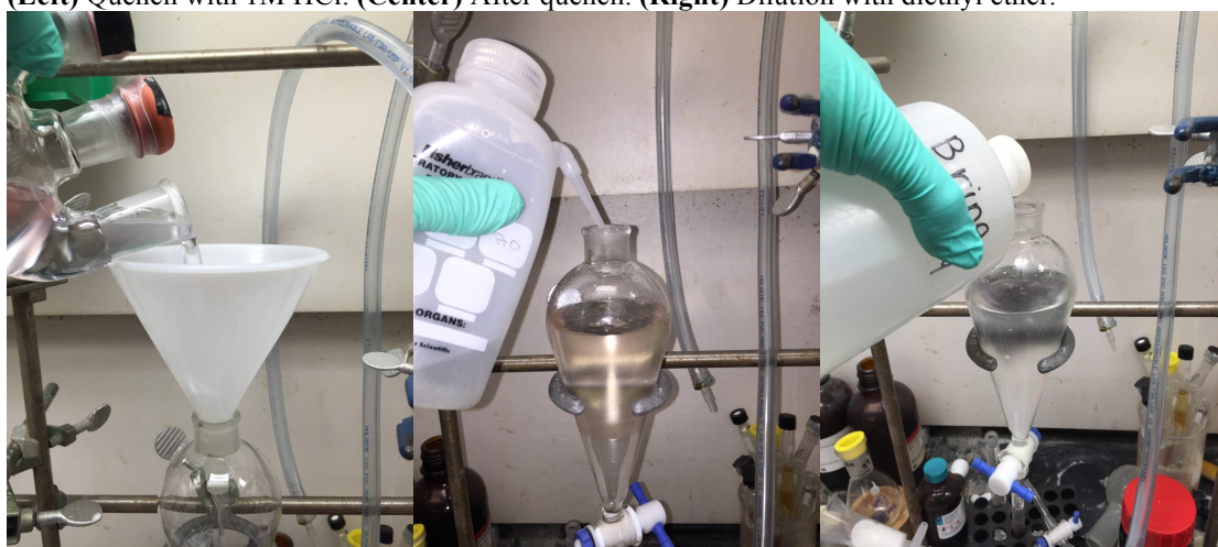
(Left) Transfer to separatory funnel. (Center) Addition of water for wash. (Right) Brine wash.
