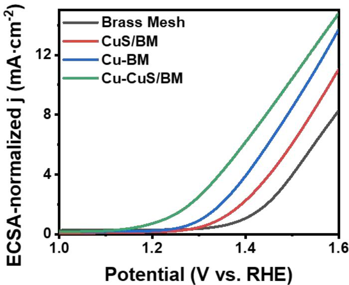
Figure S3. ECSA-normalized LSV curves of Brass Mesh, CuS/BM, Cu-BM and Cu-CuS/BM for GOR in 0.1 M KOH solution with 0.1 M glycerol.
