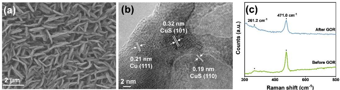
Figure S6. The SEM (a) and HRTEM (b) images of Cu-CuS/BM after long-term electrolysis. (c) The Raman spectra of Cu-CuS/BM before and after electrochemical test.
