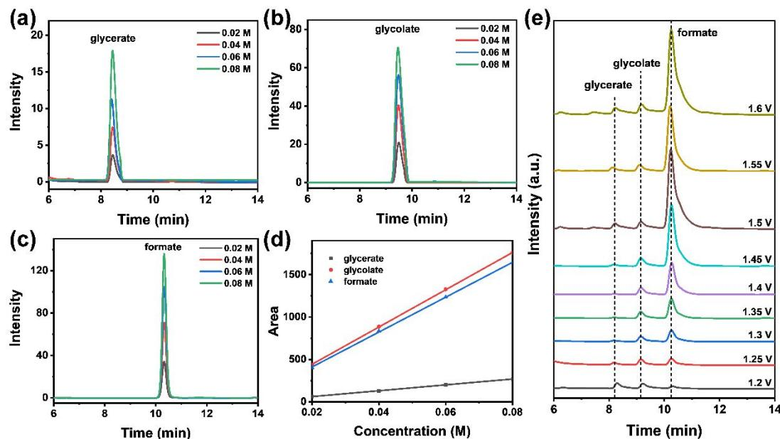
Figure S4. Standard HPLC chromatograms of glycerate (a), glycolate (b) and formate (c). (d) The standard curves of glycerate, glycolate and formate. (e) HPLC chromatograms of the reaction products from the GOR at different potentials using Cu-CuS/BM.
