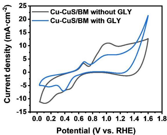
Figure S7. CV curves of the Cu-CuS/BM in 0.1 M KOH with and without 0.1 M GLY.
