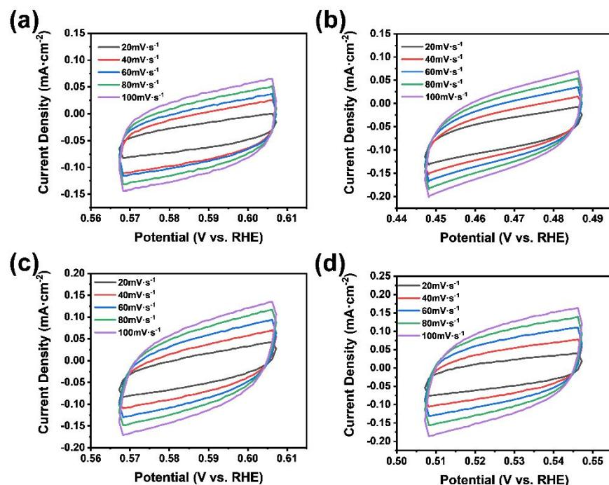
Figure S2. CV curves of the (a) BM, (b) CuS/BM, (c) Cu-BM and (d) Cu-CuS/BM at various scan rates in 0.1 M KOH in the presence of 0.1 M GLY.
