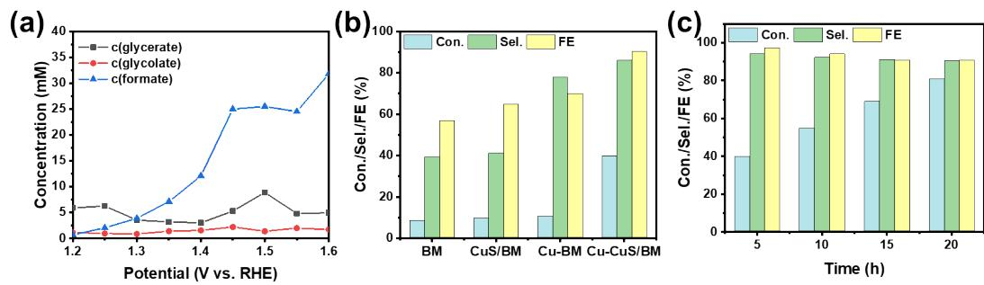
Figure S5. (a) The concentrations of the all products for GOR detected by HPLC, including glycerate, glycolate and formate. (b) The Conversion of GLY, the Selectivity and Faradaic efficiency of formate at the 1.45 V vs. RHE for GOR using the BM, CuS/BM, Cu-BM, Cu-CuS/BM. (c) The Conversion of GLY, the Selectivity and Faradaic efficiency of formate on Cu-CuS/BM after reacting 5 h, 10 h, 15 h and 20 h.
